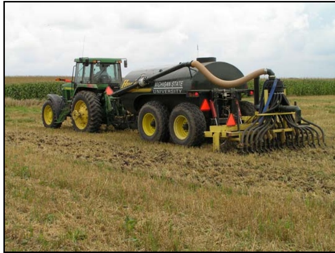
Figure 1. Seed-laden slurry was delivered through drop-tubes to the fractured soil behind each set of aeration tines. No additional seedbed tillage was used.
