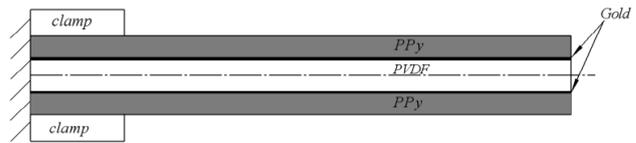
Figure 1. Geometry of the conducting polymer actuator.
