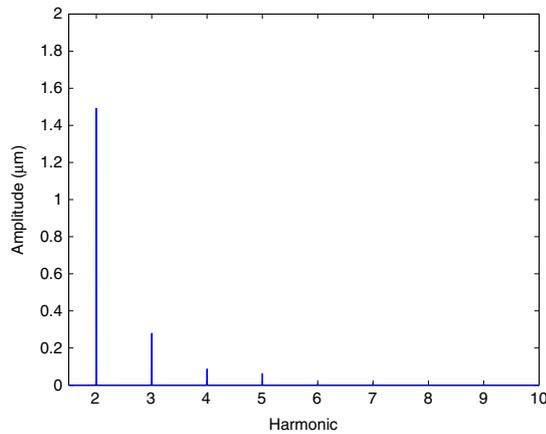
**Fig. 6.** Output spectrum for nanopositioner used in experimental studies. Input to power supply is  $3 \sin(2\pi 5) + 4V$ . Primary harmonic is not shown, but has an amplitude of  $25.2 \mu\text{m}$ .
