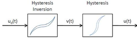
Fig. 4. Hysteresis inversion process.  $u_d$  is the desired input.
