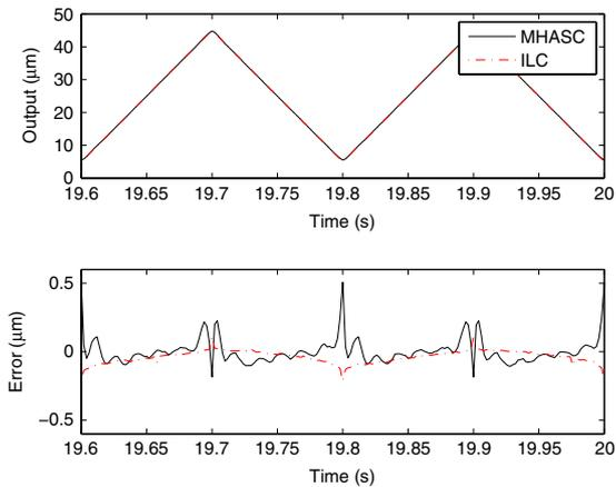
Fig. 9. Experimental results for a 5 Hz sawtooth signal.
