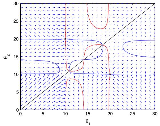
**Fig. 2.** Phase portrait of average system for a sample plant and controller. The zero level curves of  $\dot{\theta}_1$  (primarily vertical) and  $\dot{\theta}_2$  (primarily horizontal) together with the neutral axis  $\theta_1 = \theta_2$  are also plotted.
