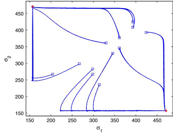
Fig. 10. Phase portrait of  $\sigma_1$  and  $\sigma_2$  for various initial conditions. Desired equilibria are marked by the stars (red, in the lower right and top left), and initial conditions are marked by squares.
