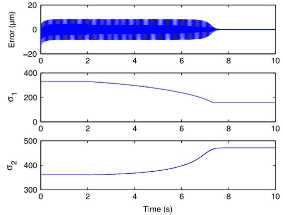
Fig. 11. Plot of tracking error and adaptation variables vs. time. Adaptation is enabled at 2 s.
