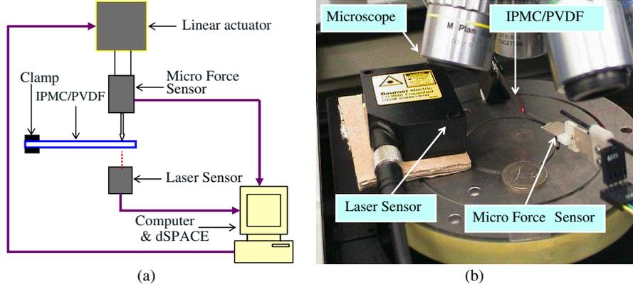
Figure 5. (a) Experimental setup for spring constant measurement; (b) picture of the experimental setup.
