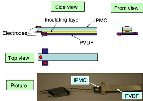
Figure 1. Design of the IPMC/PVDF composite structure.
