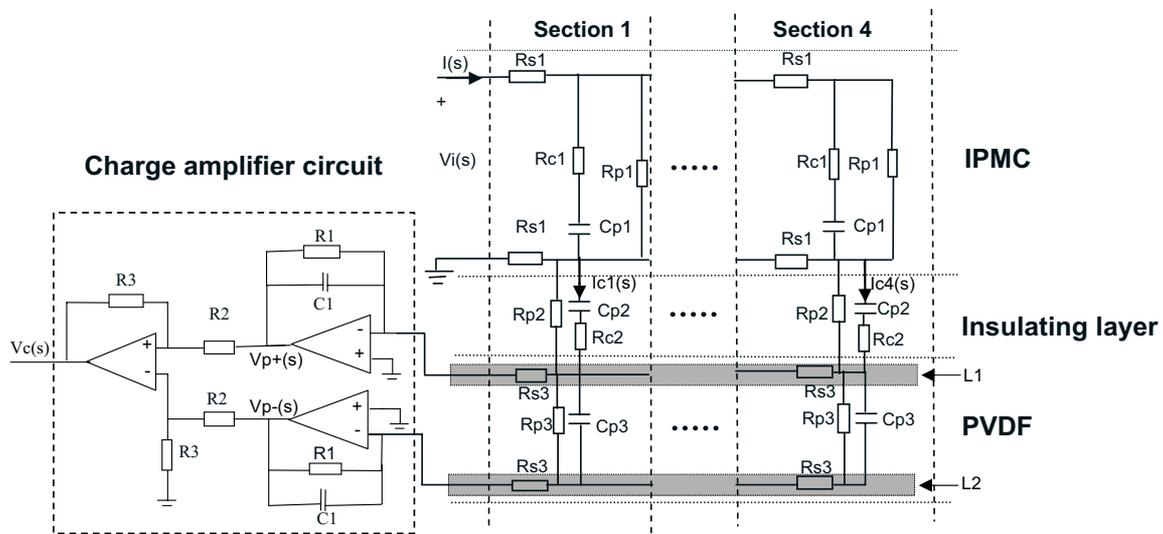
**Figure 8.** Circuit model of the IPMC/PVDF structure.
