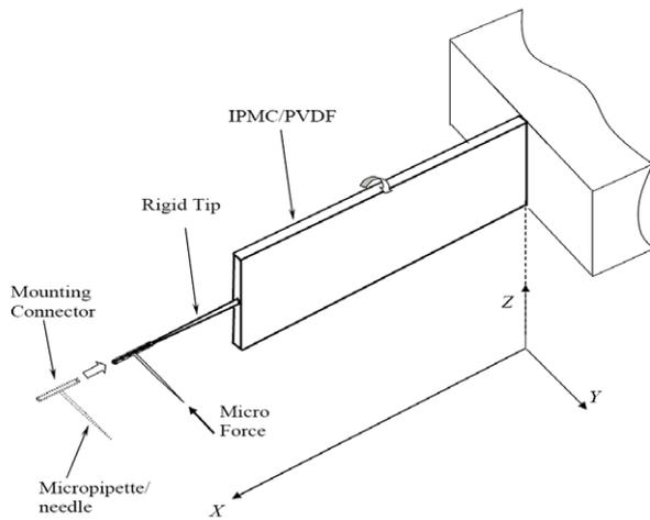
**Figure 15.** Illustration of the IPMC/PVDF micro-force injector.
