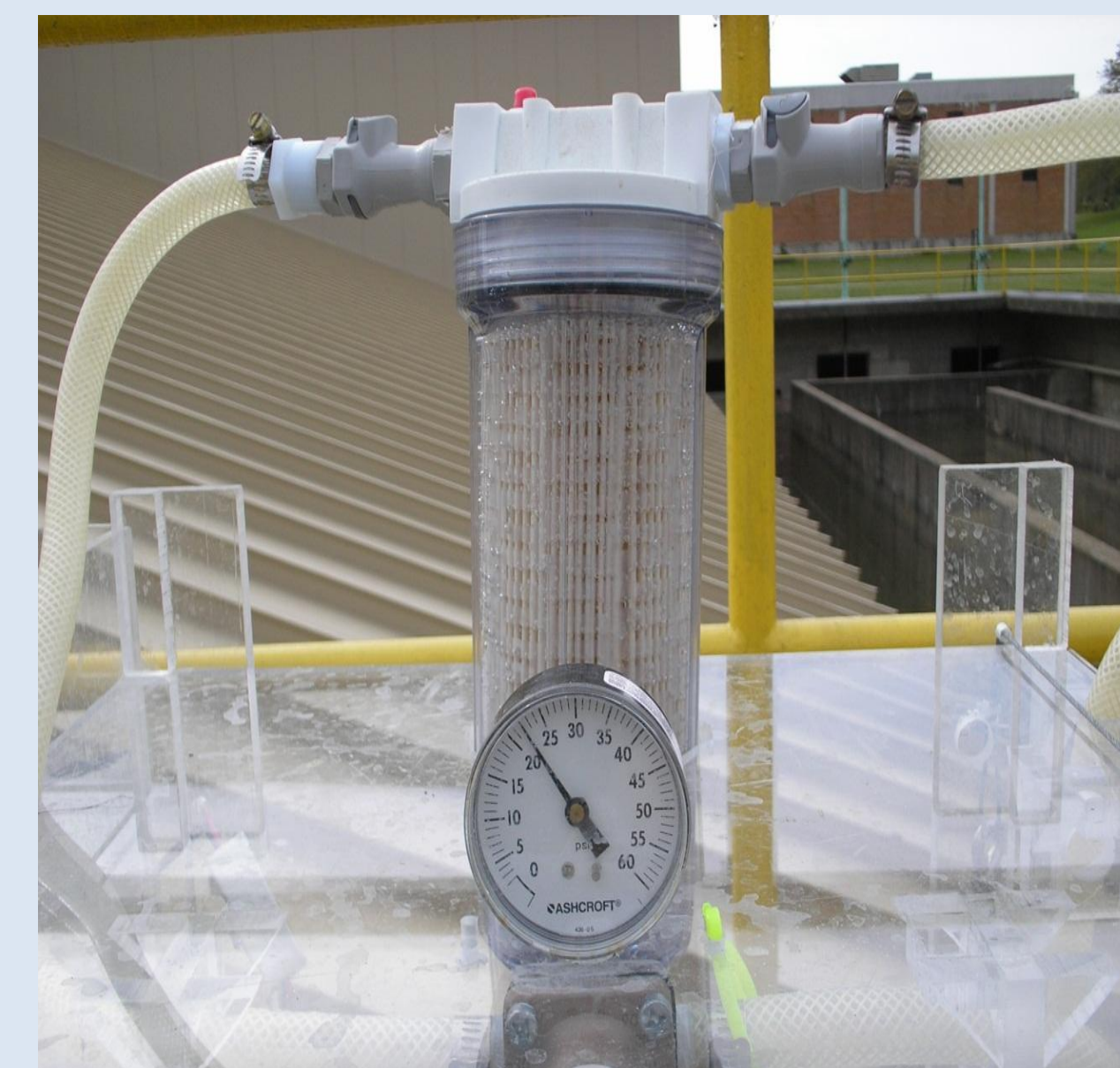
Figure 4: 1MDS filter used to sample the wastewater at each location throughout this study.
