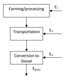
E<sub>1</sub>: includes collection and processing in order to convert to diesel
