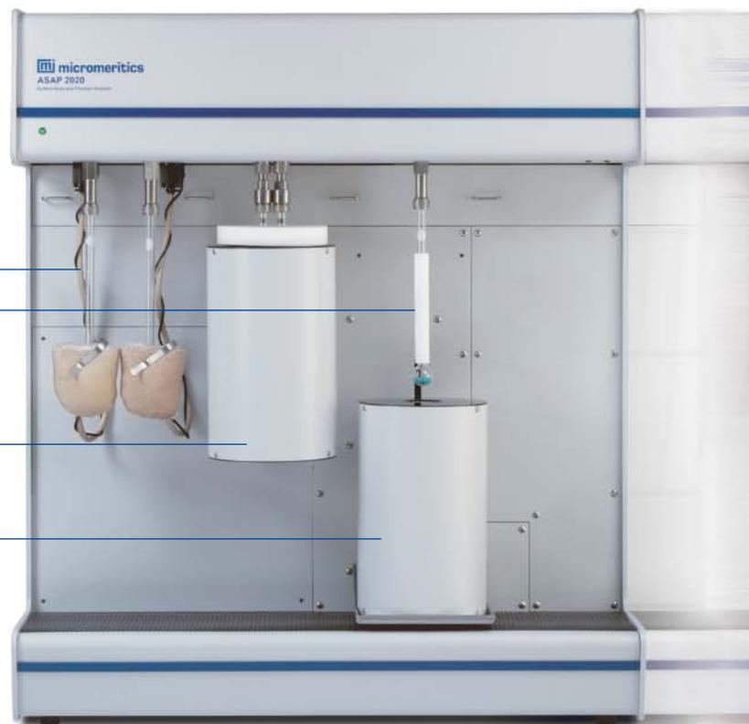
**Long-duration Dewars** combined with Micromeritics' patented **Isothermal Jackets** which are guaranteed against failure for the life of the instrument, assure a constant thermal profile along the full length of both the sample and the saturation pressure ( $P_0$ ) tubes throughout extended analyses.
