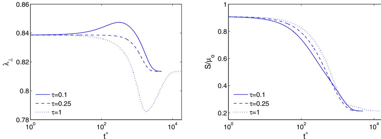
**Figure 5.** Transverse stretch  $\lambda_{\perp}$  and nominal stress  $S/\mu_0$  as a function of normalized time  $t^* = t/t_m^*$  for material I with  $\beta_f = 0.6$ . Shown is the case of a hard loading device with  $\lambda = 1.3$  and the degradation is of type MFF for all time. Here  $n_f = n_m = 2$  and the non-dimensionalized time is defined by  $t^* = t/t_m^*$ . The three curves are for  $\tau = 0.1, 0.25$ , and  $1.0$ .
