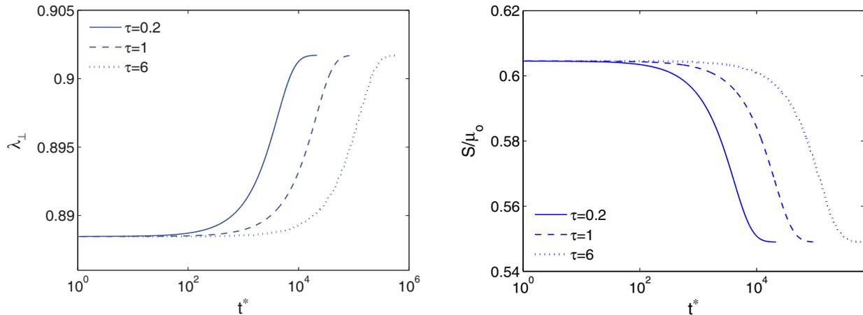
**Figure 4.** Transverse stretch  $\lambda_{\perp}$  and nominal stress  $S/\mu_0$  as a function of normalized time  $t^*$  for material I with  $\beta_f = 0.6$ . The case shown is of a hard loading device with  $\lambda = 1.2$  so that the degradation is of type FF for all time. Here  $n_f = n_m = 2$  and the non-dimensionalized time is defined by  $t^* = t/t_m^*$ . The three curves are for  $\tau = 0.2, 1, \text{ and } 6$ .
