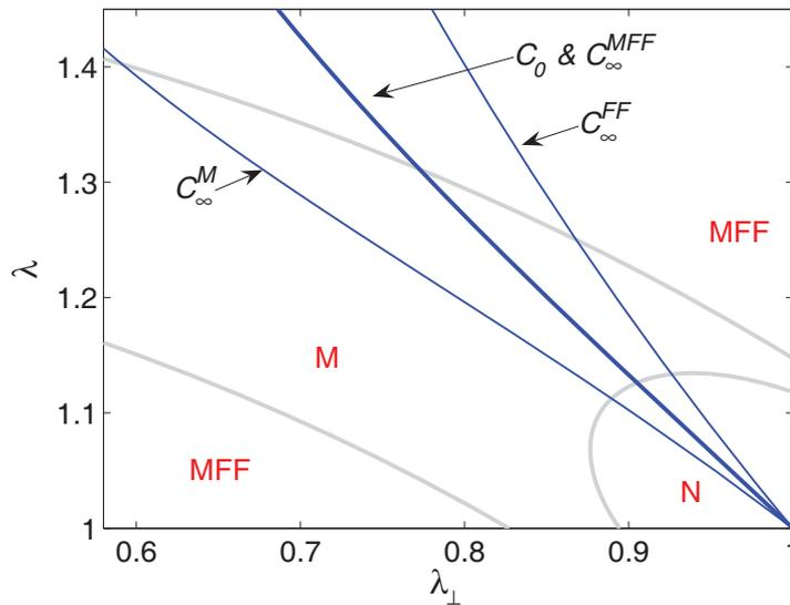
**Figure 10.** Degradation phase diagram for material 2 showing stretch state curves  $C_0$ ,  $C_\infty^M$ , and  $C_\infty^{FF}$ . For this material, since  $\beta_f = \beta_m$  the curves  $C_0$  and  $C_\infty^{MFF}$  are coincident.
