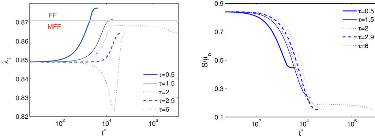
**Figure 8.** Evolution of  $\lambda_{\perp}$  and  $S/\mu_0$  with  $t^*$  for a hard loading device for material I with  $\beta_f = 0.9$  and  $\lambda = 1.2788$ . Other parameters:  $\beta_m = 0.8$ , and  $n_f = n_m = 2$ .
