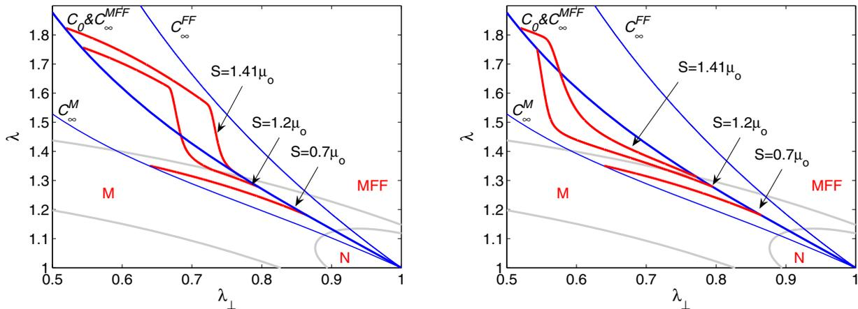
**Figure 14.** Degradation paths  $(\lambda_{\perp}(t), \lambda(t))$  for soft loading of material 2 for  $\tau = 0.001$  (left) and  $\tau = 0.01$  (right).
