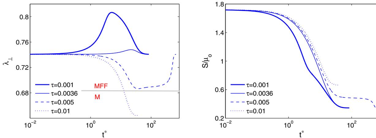
**Figure 11.** Evolution of  $\lambda_{\perp}$  and  $S/\mu_0$  with  $t^*$  for a hard loading device with material 2 and  $\lambda = 1.36$ . For this value of  $\lambda$  the degradation is initially of type MFF but may transition to type M depending on the kinetics. Four values of  $\tau$  are shown, one of which gives a transition to M degradation and three of which do not.
