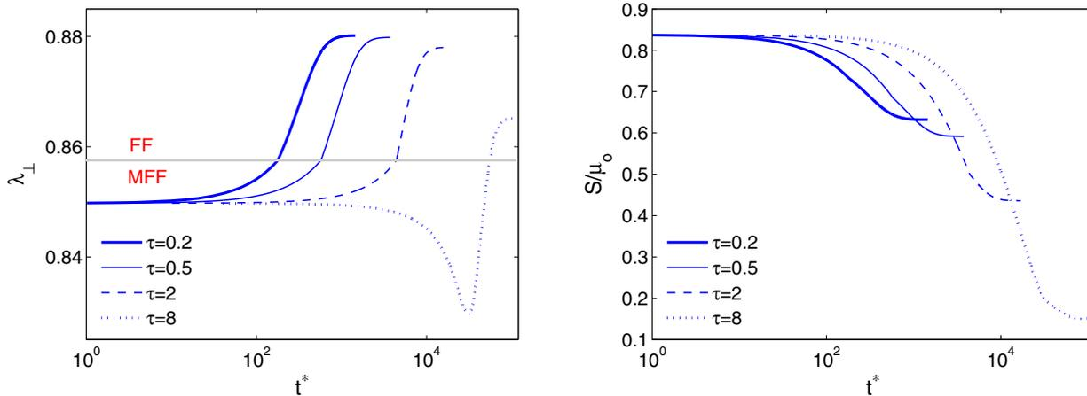
**Figure 9.** Evolution of  $\lambda_{\perp}$  and  $S/\mu_0$  with  $t^*$  for a hard loading device for material I with  $\lambda = 1.277$  and  $\beta_f = 0.9$ . Other parameters:  $\beta_m = 0.8$  and  $n_f = n_m = 2$ . Four values of  $\tau$  are used, three of which give a monotone  $\lambda_{\perp}(t)$  and one of which gives an anomalous start-up.
