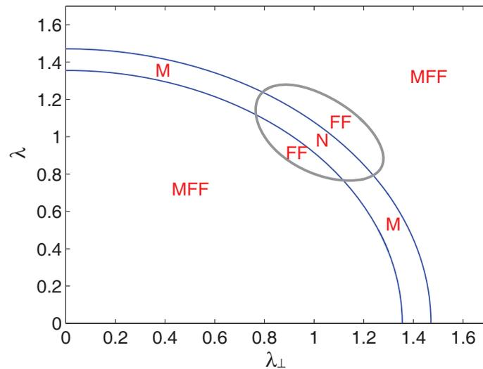
**Figure 1.** Degradation phase diagram for material 1 with  $\beta_f = 0.6$ . Note that the undeformed location  $(\lambda_{\perp}, \lambda) = (1, 1)$  is in the N region where no degradation takes place.
