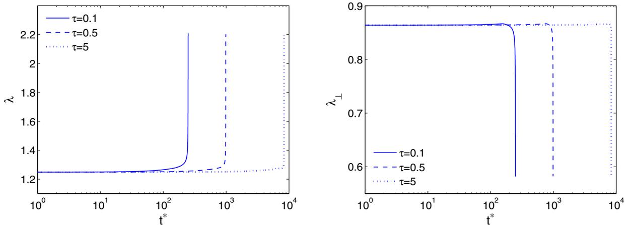
**Figure 13.** Axial stretch  $\lambda$  and transverse stretch  $\lambda_{\perp}$  as a function of normalized time  $t^* = t/t_m^*$  for material I with  $\beta_f = 0.9$  at the fixed value  $S = 0.75\mu_0$ . For this value of  $S$  the degradation is initially of type FF but then changes into type MFF. The creep-type response for three different values of  $\tau$  are shown,  $\tau = 0.1, 0.5$ , and  $5$ .
