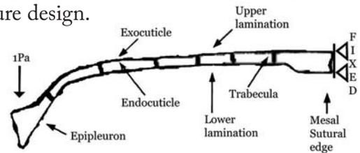
**Figure 1** Cross section of a beetle's forewing with key characteristics and finite element analysis constraints and forces labeled. Re-drawn from Ref. 1.
