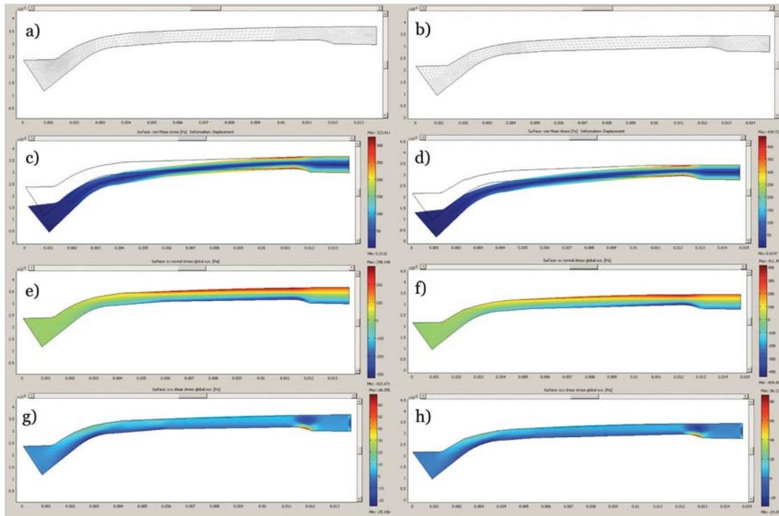
**Figure 2** Comsol Stress Analysis. The finite element mesh of the a) female forewing and b) male forewing; Von Mises stress deformation due to 1 Pa load on the c) female forewing and d) male forewing; Normal stress deformation due to 1 Pa load on the e) female forewing and f) male forewing; Shear stress deformation due to 1 Pa load on the g) female forewing and h) male forewing.
