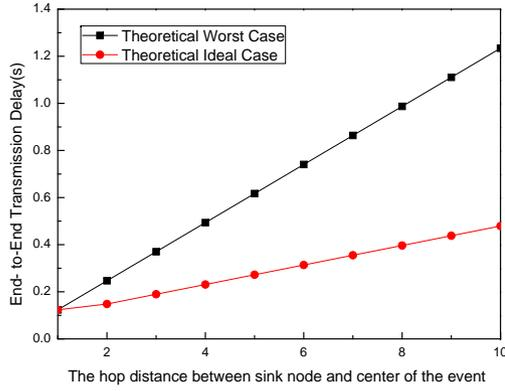
**Figure 4.** The end-to-end transmission delay in multi hops. There are 20 contending nodes in the source node.
