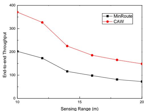
**Figure 8.** Network throughput with varying event sensing range
