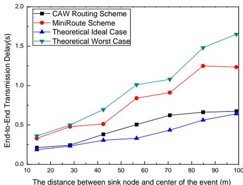
**Figure 6.** Average packets end-to-end transmission delay with varying burst event location
