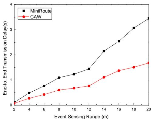
**Figure 7.** Average packet end-to-end transmission delay with varying event sensing range
