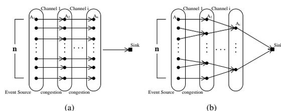
**Figure 1.** The link layer congestion: (a) General distributed routing algorithms that may lead to congestion in subsequent forwarding; (b) Illustration of the CAW routing algorithm
