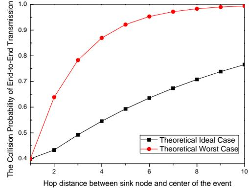
Figure 3. The end-to-end collision probability in multi hops. There are 20 contending nodes in the source node.
