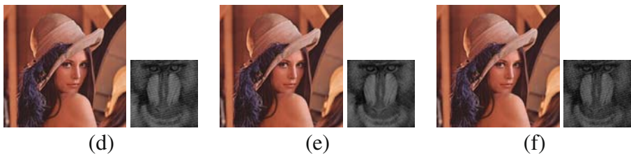
Fig. 11 Frequency domain example 3—cropped watermarked images and the extracted watermarks: d Cropped the lower 1/3 (MSE = 0.6111, PSNR = 50.2696), e cropped the right 1/3 (MSE = 0.6142, PSNR = 50.2479), f cropped the 50 outside pixels (MSE = 0.5424, PSNR = 50.7873)
