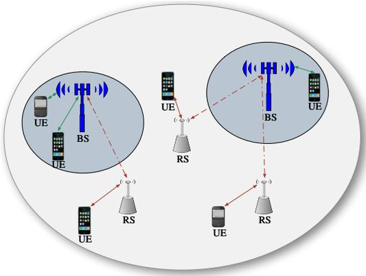
Fig. 1. The proposed relay-assisted network architecture.
