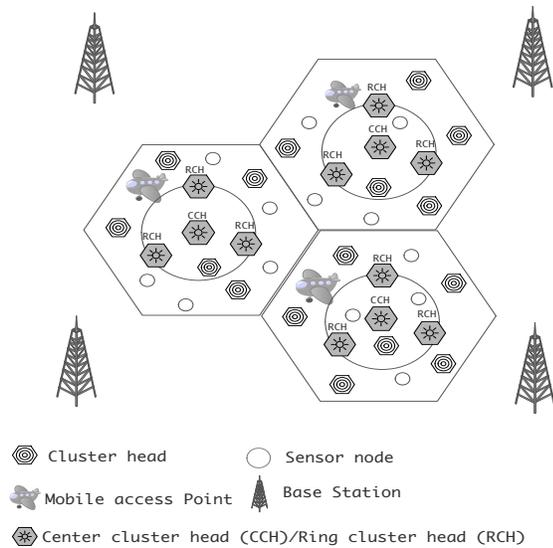
Fig. 1. Proposed MC-WSN architecture.
