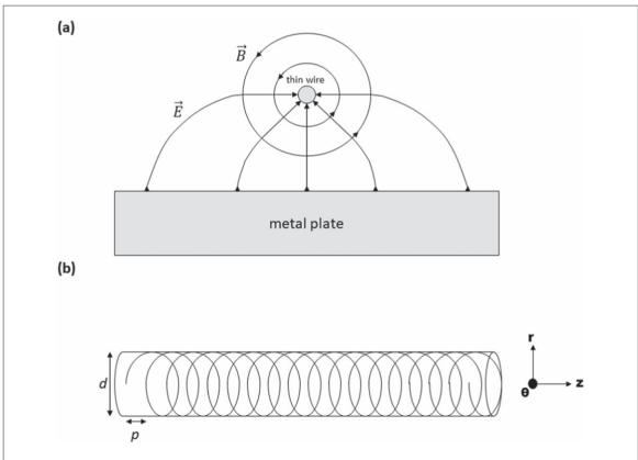
**Figure 3.** (a) Depiction of the TEM fields of a thin wire over a perfectly conducting metal plate. (b) The formation of a helix TWT from 'wrapping' the set-up in (a).
