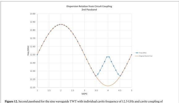
**Figure 12.** Second passband for the sine waveguide TWT with individual cavity frequency of 12.5 GHz and cavity coupling of c = 0.03.
