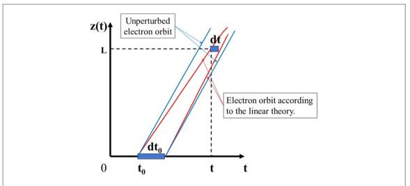
Figure 5. An (exaggerated) illustration of harmonic generation due to orbital crowding. Crowding in the linear orbits may lead to harmonic current generation, as shown in klystron theory [3] and TWT theory [43].
