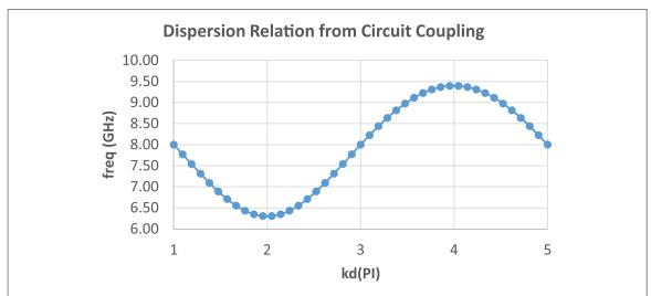
**Figure 11.** Dispersion relation for a 20 cavity sine waveguide TWT constructed from a coupled cavity approach. Individual cavities have a resonant frequency of 8 GHz and the dimensionless coupling between the cavities is c = 0.19.
