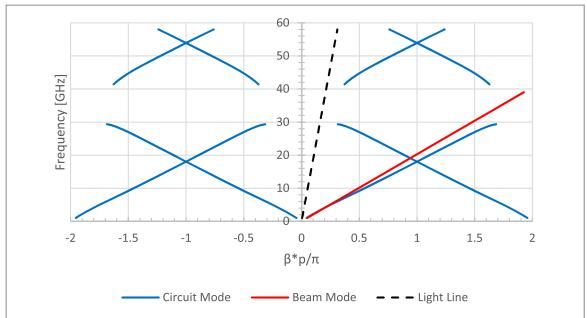
**Figure 4.** Dispersion diagram for a tape helix showing several circuit modes ( $\beta = \Gamma_0$ , blue) and the beam mode ( $\beta = \frac{\omega}{v_0}$ , red). Also included in the Figure is the light line ( $\beta = \frac{\omega}{\epsilon}$ , black, dashed).
