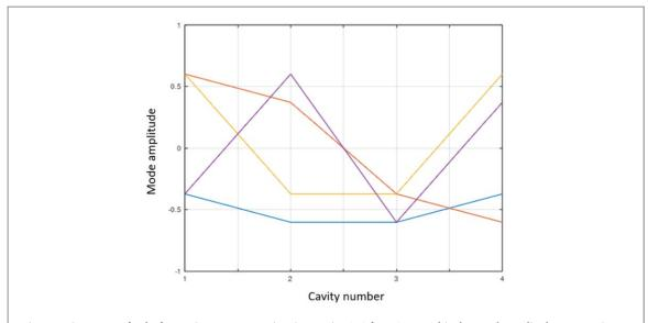
**Figure 8.** Eigenvectors for the four cavity system roots given in equation (13) from Octave. This plots mode amplitude versus cavity number. Thus, the horizontal axis gives the axial location of the field.
