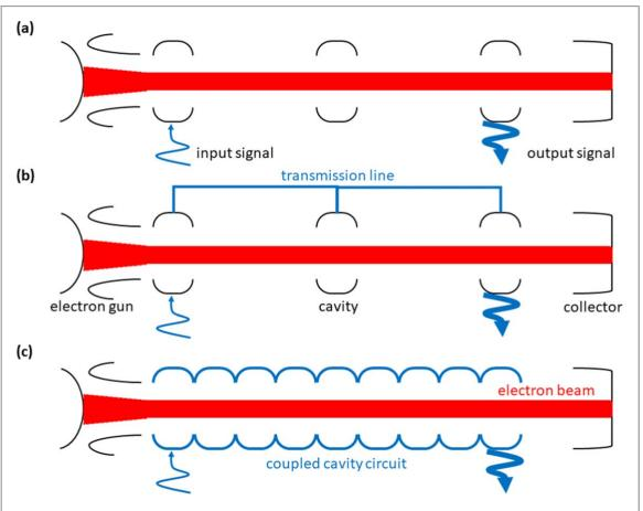
**Figure 1.** Schematic diagram showing the evolution of a multi-cavity klystron (a) to a traveling-wave tube amplifier (c). (b) shows the multi-cavity klystron with its cavities coupled to a common transmission line.
