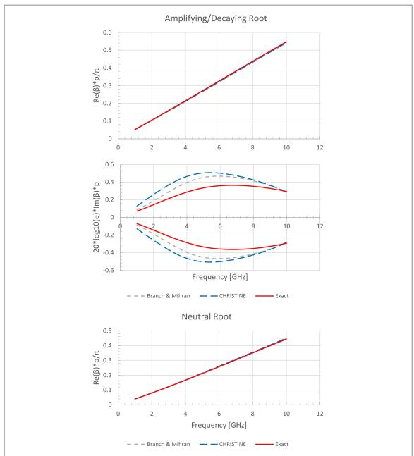
Figure 6. Plot of the three roots (propagation constant  $\beta$ ) as determined from: Pierce theory with Q modeled by Branch and Mihran (gray, dashed) [14], Pierce theory with Q modeled by the sheath helix model as used by CHRISTENE [44] (blue, dashed), and the exact dispersion relation (red, solid) as a function of input signal frequency. Image adapted from [39].
