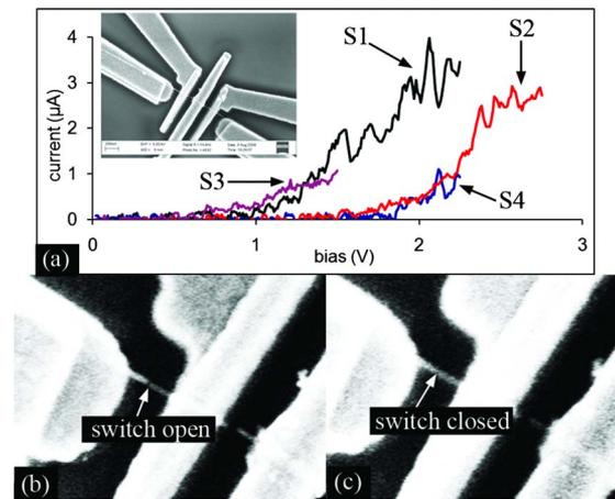
FIG. 2. (Color online) Switching results. (a) I-V plots of switches with low turn-on bias (0.8 to 2 V in this case). The engineered NT is shown in inset. [(b) and (c)] SEM images of a device in the open and closed configurations.
