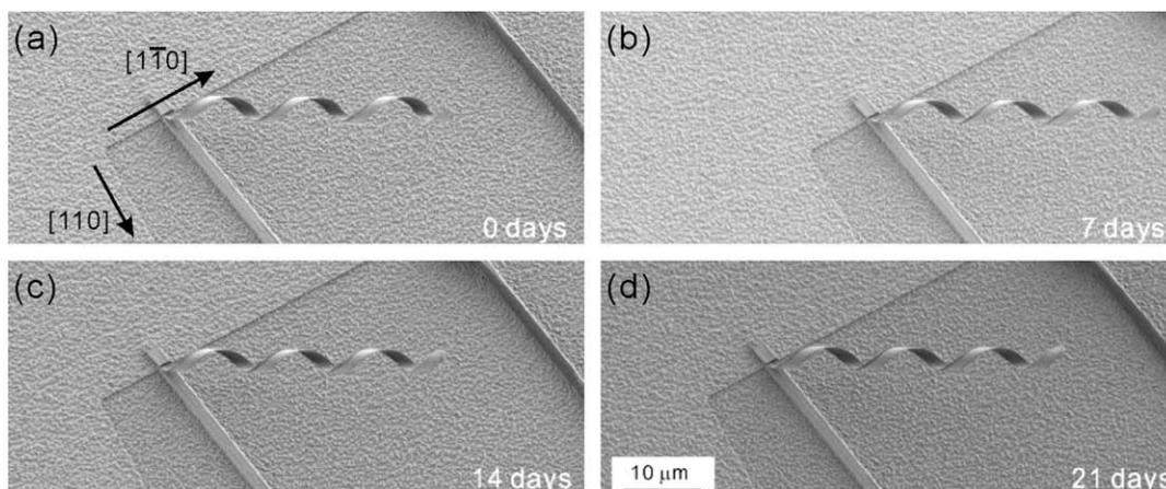
Fig. 1. The as-fabricated sample is exposed to air for several weeks. The sample is inspected by FESEM with the same viewing orientation. All four images have the same scale bar. The helix was prepared on a GaAs (001) wafer with a trilayer, i.e. InGaAs/GaAs/Cr (11/16/15 nm). The orientation of the ribbon-like patterned mesa has 10° deviation from the [110].
