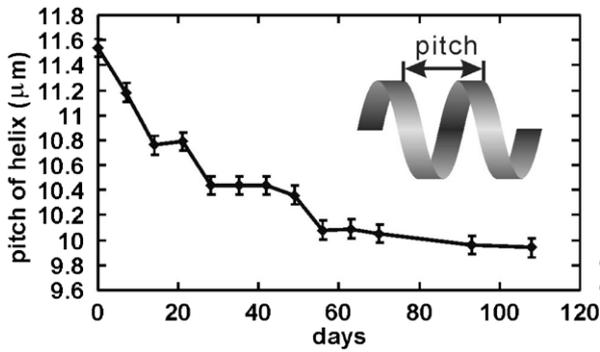
**Fig. 3.** Dependence of helix pitch with time, the helix has three turns and has the same stacked layers as the helix shown in Fig. 1. The inset shows the pitch of the helix, which means the translational distance along the helix axis with one complete helix turn.
