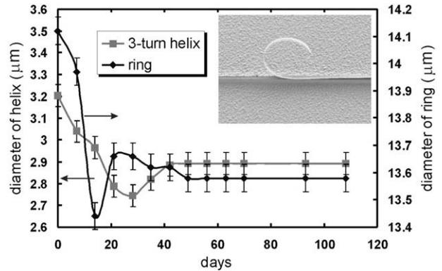
Fig. 2. Dependence of diameter of helical nanobelts on time. Both helical and ring structures have InGaAs/GaAs bilayers with thickness of (11/16 nm). Helical and ring structures are coated with 15 nm and 30 nm thick Cr, respectively.
