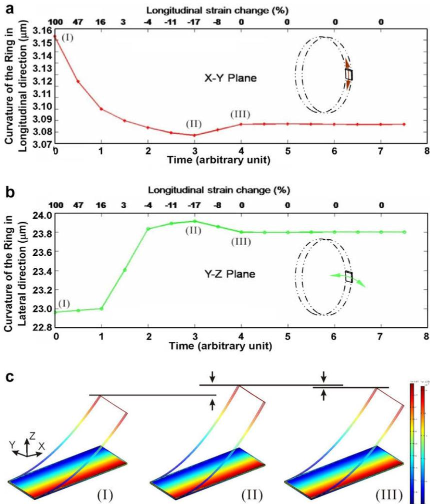
**Fig. 4.** FEM results of curvature evolution in biaxial directions for ring structure. (a) Curvature change in the longitudinal axis (X–Z plane) of the ribbon due to stress relaxation. (b) Curvature change in the transversal axis (Y–Z plane) of the ribbon due to stress relaxation. (c) Curvature radius to stress states of the ribbon for (I) (II) (III) in (a). The length and the width of the ribbon for simulation are  $4 \mu\text{m}$  and  $1.5 \mu\text{m}$ , respectively.
