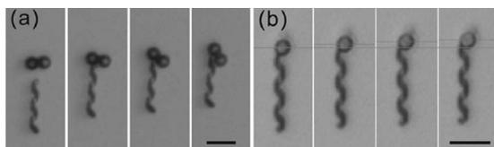
FIG. 5. (a) Two polystyrene microspheres are rotated  $70^\circ$  by a  $29\ \mu\text{m}$  long InGaAs/GaAs/Cr ABF pushing on one of the microspheres. The optical-microscope image sequence represents 2 s of elapsed time. (b) The microsphere is pushed for a radius length by the ABF within 1 s. The scale bars are  $15\ \mu\text{m}$ .
