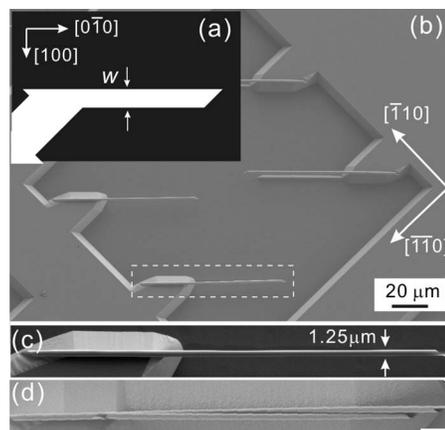
FIG. 1. (a) The initial mesa pattern used to fabricate freestanding SiGe/Si microtubes. The main scrolling directions of the bilayer are  $[100]$  and  $[-100]$ . (b) FESEM image of an array of SiGe/Si microtubes. The regions in the white dashed lines are magnified in (c). (d) FESEM image of a twin tube, the scale bar is  $5 \mu\text{m}$ .
