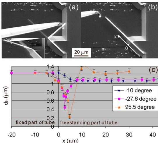
FIG. 3. (Color online) Bending tests of freestanding SiGe/Si microtubes. (a) A SiGe/Si microtube is buckled locally with a bending angle of  $95.5^\circ$  and  $-27.6^\circ$  by the manipulator probe. (b) The tube recovers to its original shape after the probe is removed. (c) The curves show that the local diameter of tube ( $d_h$ ) from a top-view SEM image depends on the tube  $x$  axis.
