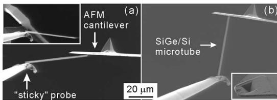
FIG. 2. Nanorobotic manipulation of a freestanding SiGe/Si microtube. (a) Placing a microtube on the backside of an AFM cantilever. Inset: Cutting of a microtube from the Si substrate. (b) Rotating a microtube on an AFM cantilever. Inset: AFM cantilever with a hole on its backside.
