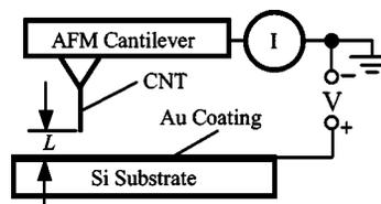
FIG. 1. Configuration of CNT-emitter EBID system.
