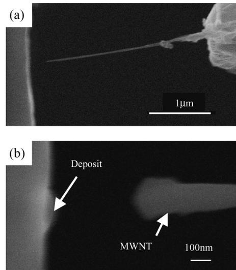
FIG. 4. EBID through MWNT electron emitter: (a) before EBID and (b) after EBID.
