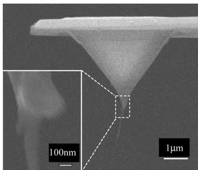
FIG. 3. CNT emitter (inset shows the EBID deposit).
