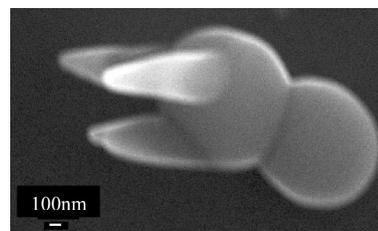
FIG. 5. EBID through conventional EBID (acceleration voltage: 15 kV, emitter current:  $106 \mu\text{A}$ , deposition time: 3 min  $\times$  4 times/finger, and base:  $\phi 1 \mu\text{m}$  polystyrene bead).
