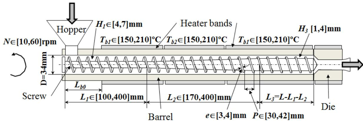
Figure 6: Single screw extruder for case study 2.
