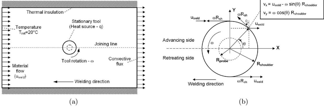
Figure 9: (a) 2-D Eulerian steady state thermal model for case study 3. (b) Mathematical modeling of the flow field under the tool shoulder in detail.
