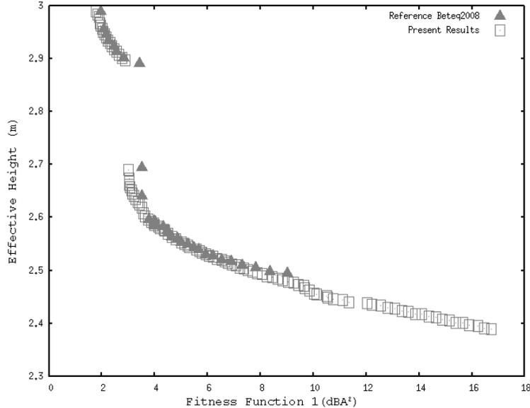
Figure 2: Accumulated non-dominated solutions in objective space for case study 1.
