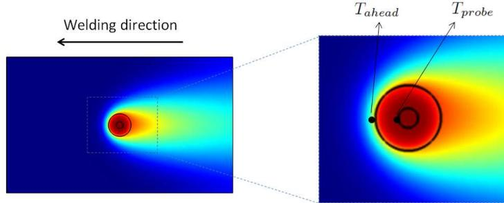
Figure 10: Thermal field at steady-state conditions for case study 3.
