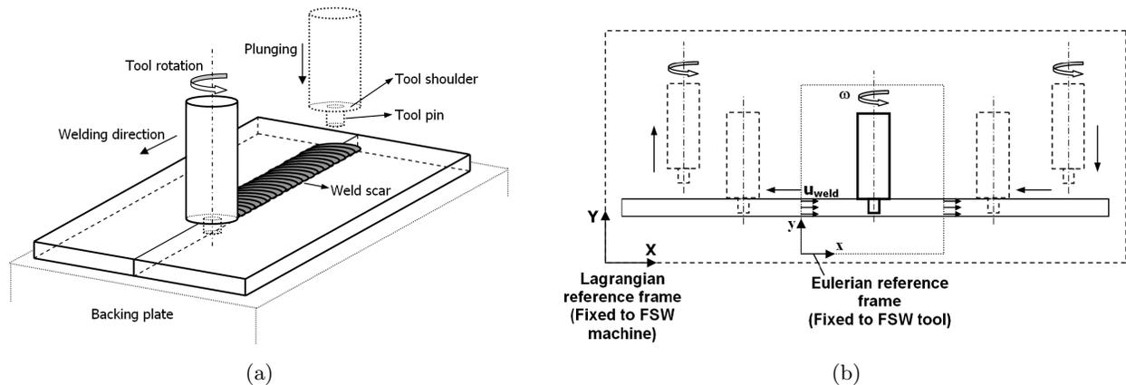
Figure 8: (a) Schematic view of the FSW process for case study 3. (b) Lagrangian (global) approach versus Eulerian (local) approach for simulation of the FSW process.
