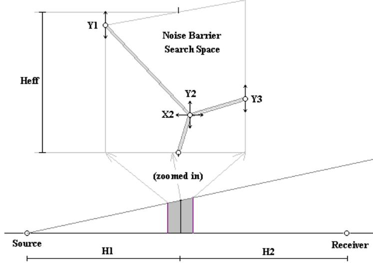
Figure 1: Y-noise barrier shape design search space for case study 1.
