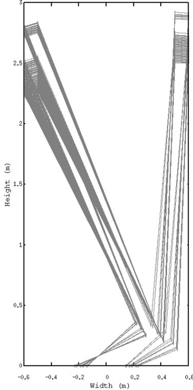
Figure 3: Accumulated non-dominated noise barrier designs (variable space) for case study 1.
