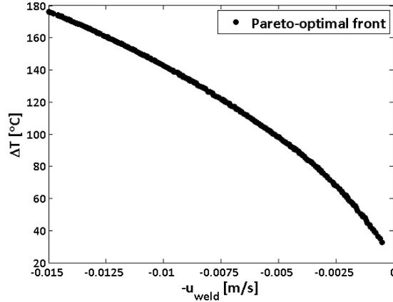
Figure 11: Pareto-optimal front for the FSW problem ( $f_1$ :  $Min. -u_{weld}$ ,  $f_2$ :  $Min. \Delta T$ ) containing 287 non-dominated solutions for case study 3.
