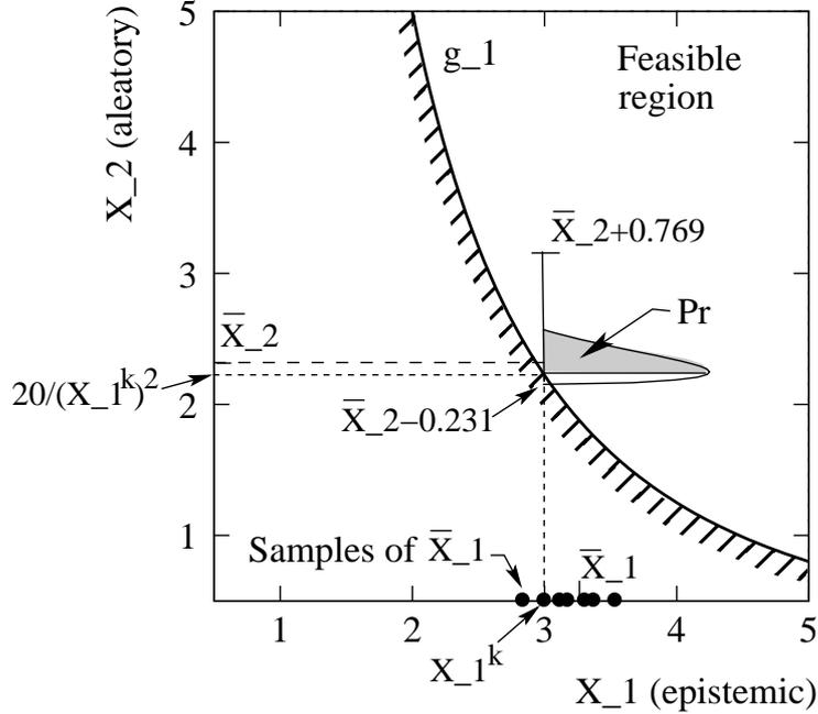
Figure 3: Computation of  $Pr [g_1(X_2) \leq 0 | X_1^k]$  for  $g_1$  constraint on a hypothetical  $(\bar{X}_1, \bar{X}_2)$  solution for a particular sample of  $\bar{X}_1 (= \bar{X}_1^k)$  is illustrated.
