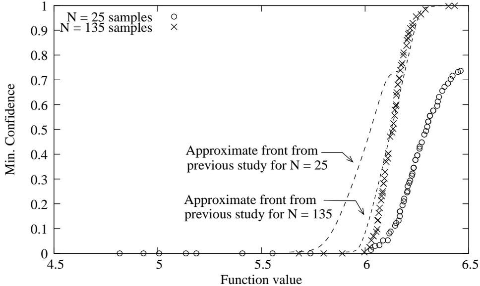
Figure 4: Trade-off of confidence level vs. objective function value for fixed reliability (95%) for all constraints (two variable numerical problem). Results are compared with that of a previous study [17].
