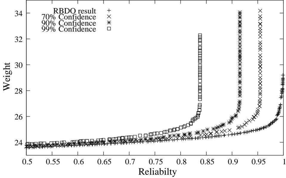
Figure 11: Trade-off fronts obtained using 25 samples of  $X_5$ ,  $X_8$  and  $X_9$  with different confidence levels (modified car side impact problem).
