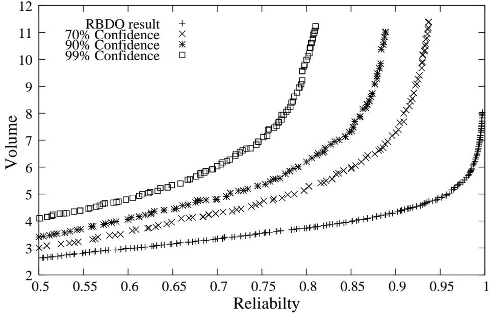
Figure 13: Trade-off fronts obtained using 25 samples of  $d$ ,  $G$  and  $S$  for different confidence levels (spring design problem).
