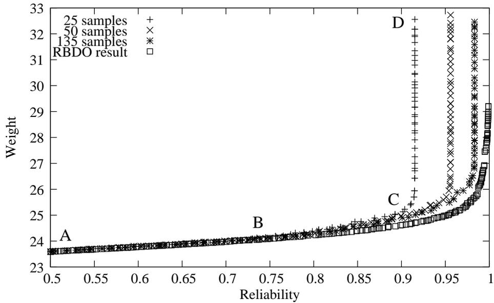
Figure 9: Trade-off fronts obtained using different number of samples of  $X_5$  with 90% confidence (car side impact problem).
