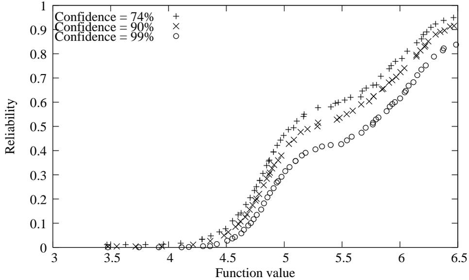
Figure 6: Comparison of Bayesian reliability fronts for different confidence values and 25 samples of  $X_1$  (two variable numerical problem).
