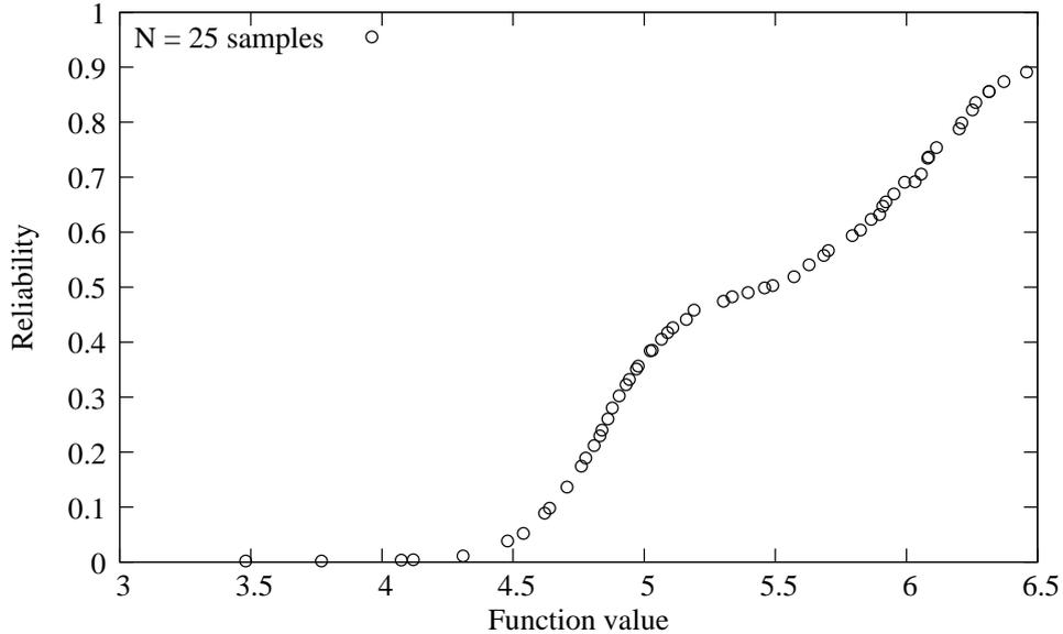
Figure 5: Bayesian reliability front for 95% confidence in each constraint and 25 samples of  $X_1$  (two variable numerical problem).
