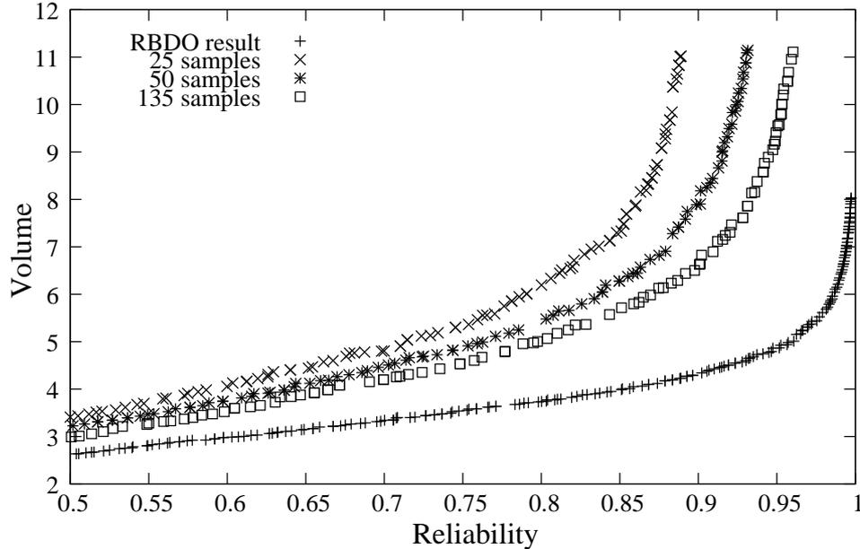
Figure 14: Trade-off fronts obtained using different number of samples of  $d$ ,  $G$  and  $S$  for 90% confidence (spring design problem).
