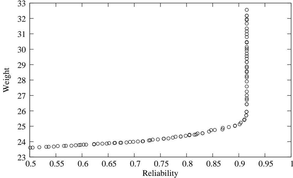
Figure 7: Weight versus reliability trade-off front using 25 samples of  $X_5$  with 90% confidence (car side impact problem).
