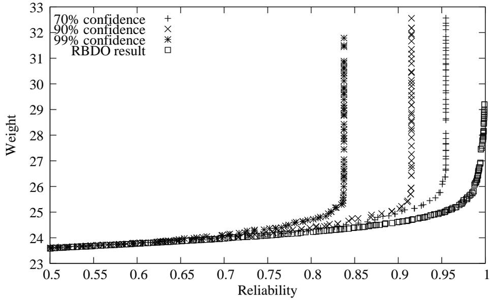
Figure 8: Trade-off fronts obtained using 25 samples of  $X_5$  with different confidence levels (car side impact problem).
