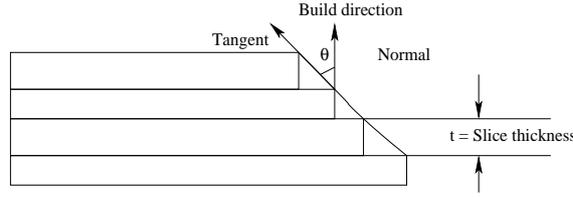
Figure 1: Showing how  $Ra$  is computed for a layer based on  $\theta$ .
