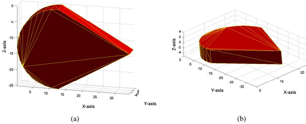
Figure 14: (a) Min.  $Ra$  orientation for Pie  $(\theta_x, \theta_y) = (90.0^\circ, 90.0^\circ)$ ,  $(Ra, T) = (42.39, 54.0)$ . (b)  $L_2$ -metric decision choice orientation for Pie  $(\theta_x, \theta_y) = (172.8^\circ, 0.72^\circ)$ ,  $(Ra, T) = (43.51, 20.0)$ .
