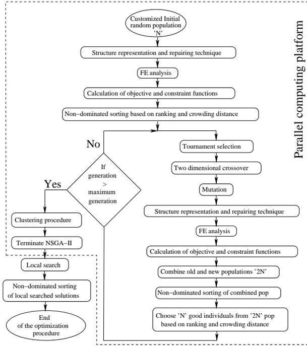
Fig. 3. A flow chart of customized NSGA-II algorithm
