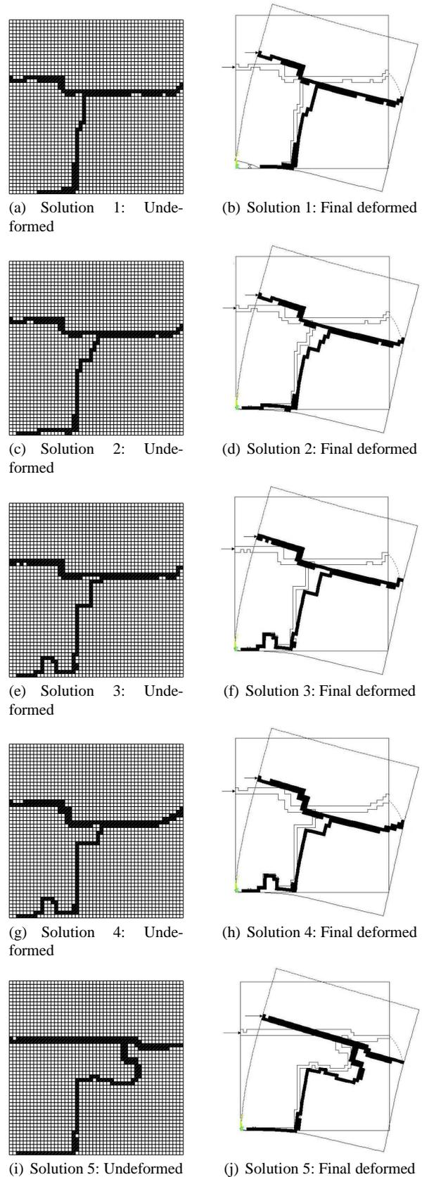
**Fig. 11** Non-dominated topologies of compliant mechanisms generating curvilinear path.
