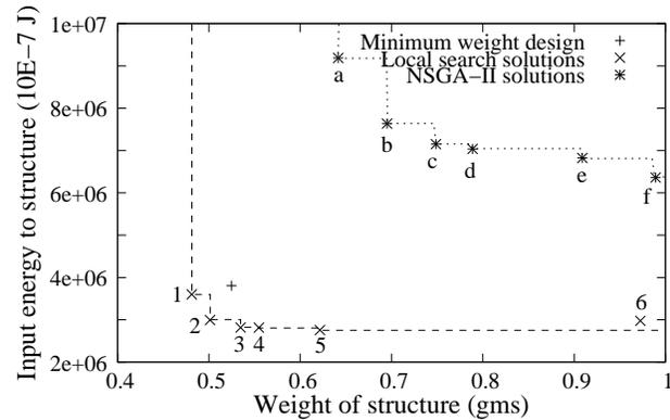
**Fig. 10** NSGA-II solutions before and after the local search and compared with the single-objective 'minimum-weight' design.
