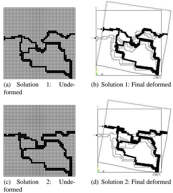
**Fig. 16** Non-dominated topologies of compliant mechanisms generating straight line path.
