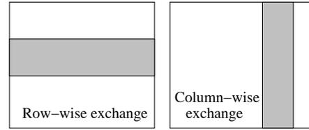
**Fig. 7** A two dimensional crossover which swaps a patch of row/column between two parent solutions.
