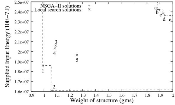
**Fig. 15** NSGA-II and local search solutions for compliant mechanisms tracing straight line path.
