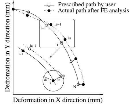
Fig. 2. An actual path traced by a structure after FE analysis and the prescribed path.
