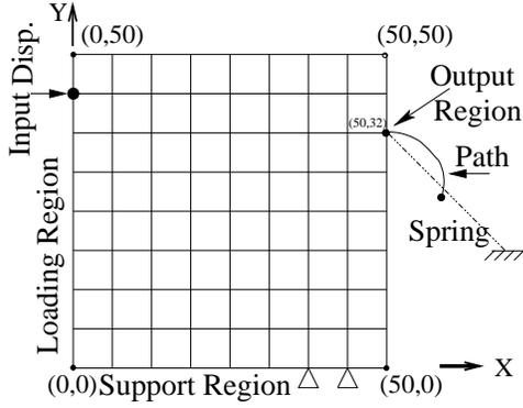
Fig. 1. Design space with loading, output and support regions.
