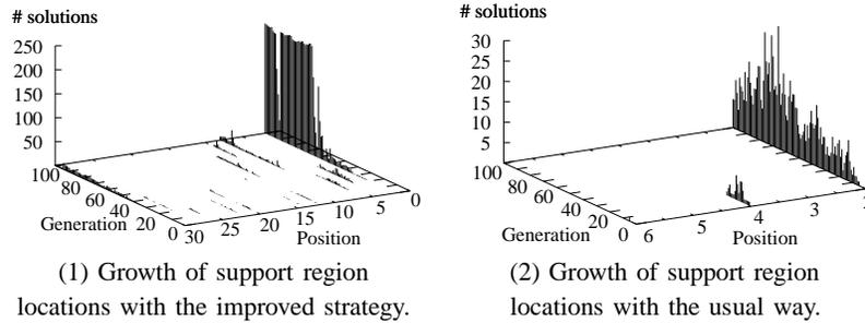
Fig. 13. Progress of non-dominated feasible solutions during NSGA-II run. Some diversity is maintained in the improved strategy
