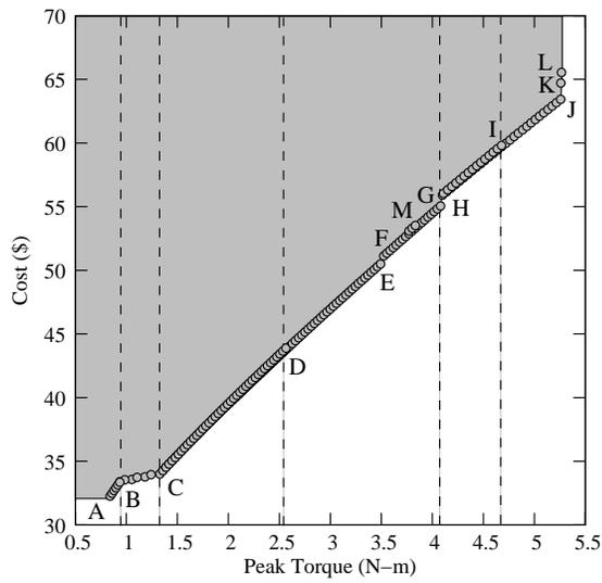
Fig. 3. Pareto-optimal Front for the original BDCPM motor design problem.
