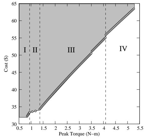
Fig. 9. Pareto-optimal front with main-stream solutions.
