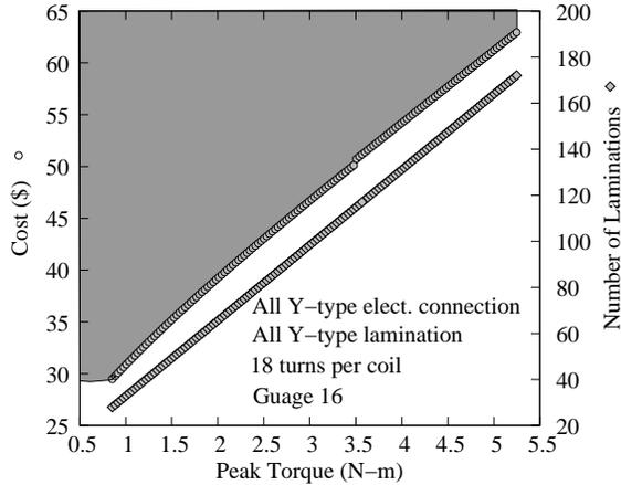
Fig. 14. Pareto-optimal front and variation of variables for the further modified problem.
