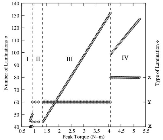
Fig. 10. Number and type of laminations for the partial Pareto-optimal front.
