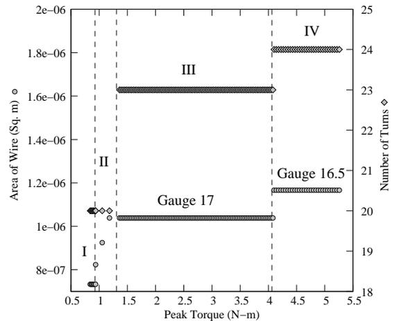
Fig. 11. Area of wire and number of turns for the partial Pareto-optimal front.
