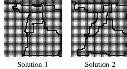
Fig. 13. Near minimum-weight topologies of compliant mechanisms tracing straight line path.
