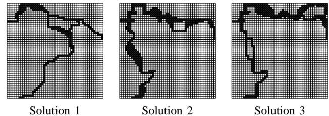
Fig. 9. Near minimum-weight topologies of compliant mechanisms tracing curvilinear path.
