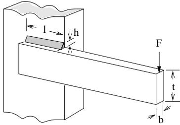
Fig. 19. The welded beam design problem.
