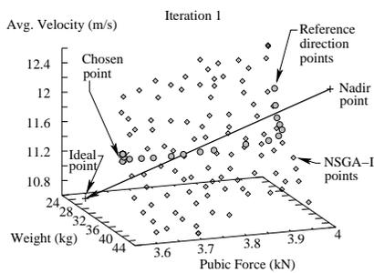
**Figure 13: First iteration of RD-NSGA-II procedure on the car side impact problem.**
