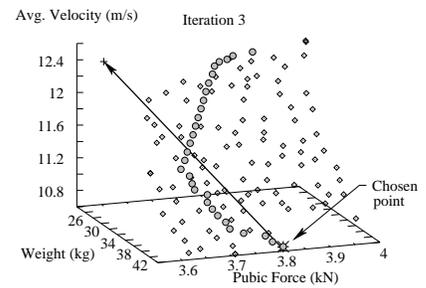
**Figure 15: Third iteration of RD-NSGA-II procedure on the car side impact problem.**
