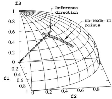
Figure 6: Step 2 of proposed algorithm in DTLZ2 with one reference direction.
