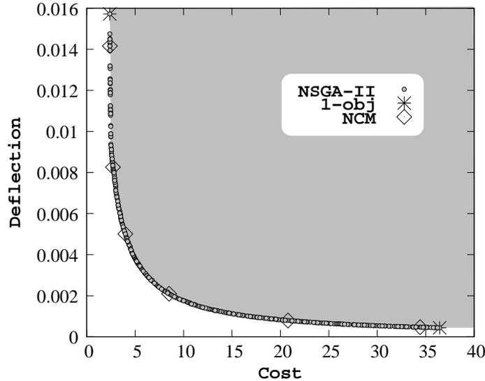
**Fig. 10.** NSGA-II solutions are shown for the welded-beam design problem.
