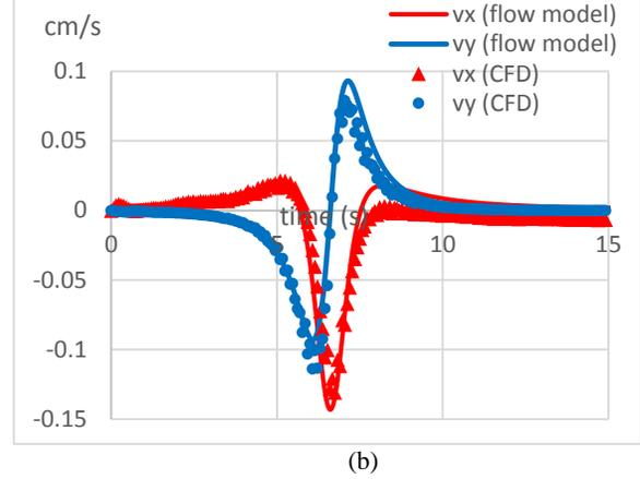
Figure 7. CFD simulation a) setup b) CFD and flow model results.
