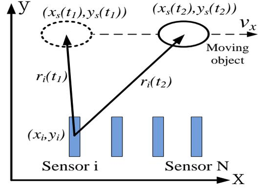
Figure 1. Illustration of the tracking of a moving object
