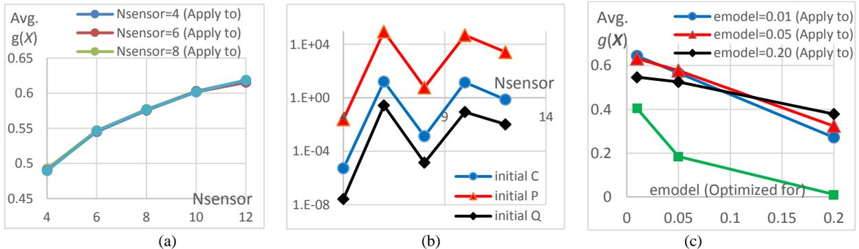
Figure 4. a) Average fitness of 50 designs evaluated when  $\varepsilon_{\text{model}}=0.05$ , and  $z^*(0.05, N_{\text{sensor}})$  is applied. b)  $z^*(0.05, N_{\text{sensor}})$  for  $\varepsilon_{\text{model}}=0.05$ . c) Average fitness of 50 designs when  $N_{\text{sensor}}=8$ , and  $z^*(\varepsilon_{\text{model}}, 8)$  is applied as the initial values of the EKF.
