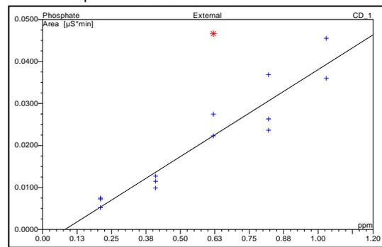
The MDL for total phosphorus was 0.24 +/- 0.03 mg/L with 95 percent confidence. The standard curve for total phosphorus is shown in Figure 3. The total phosphorus correlation coefficient was 94.7 percent, 5.1% lower than the orthophosphorus due to the nature of the digestion process.
