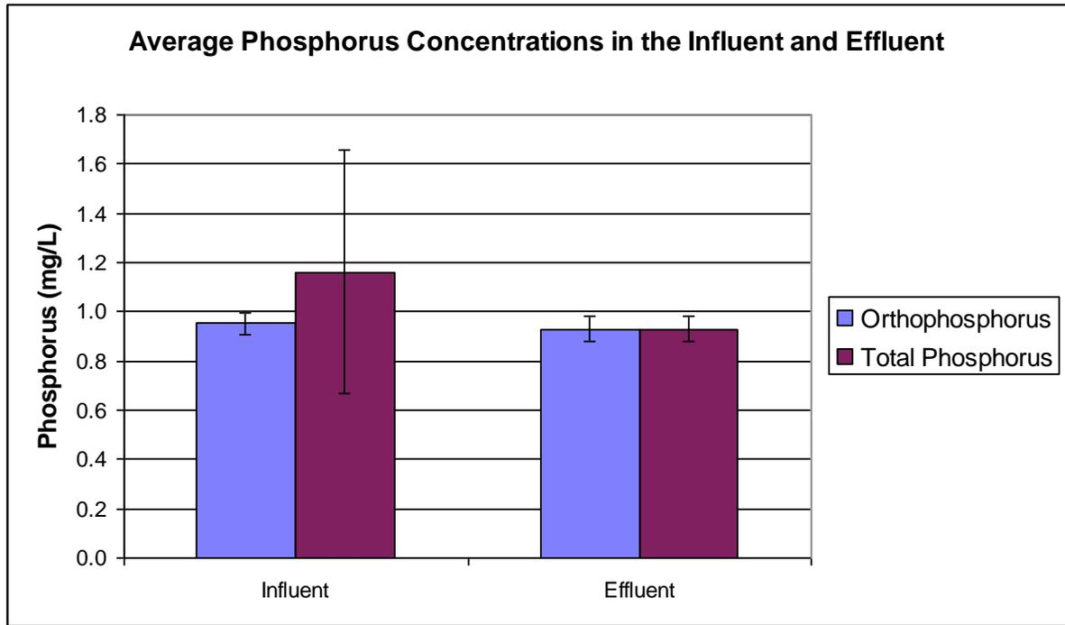
There was a high variability of total phosphorus in the influent samples with only two samples showing particulate phosphorus. This is most likely due to settling of particulate matter during storage. 100 percent of the phosphorus detected in the effluent samples was orthophosphorus, indicating that membrane filtration removed 100 percent of particulate phosphorus.
