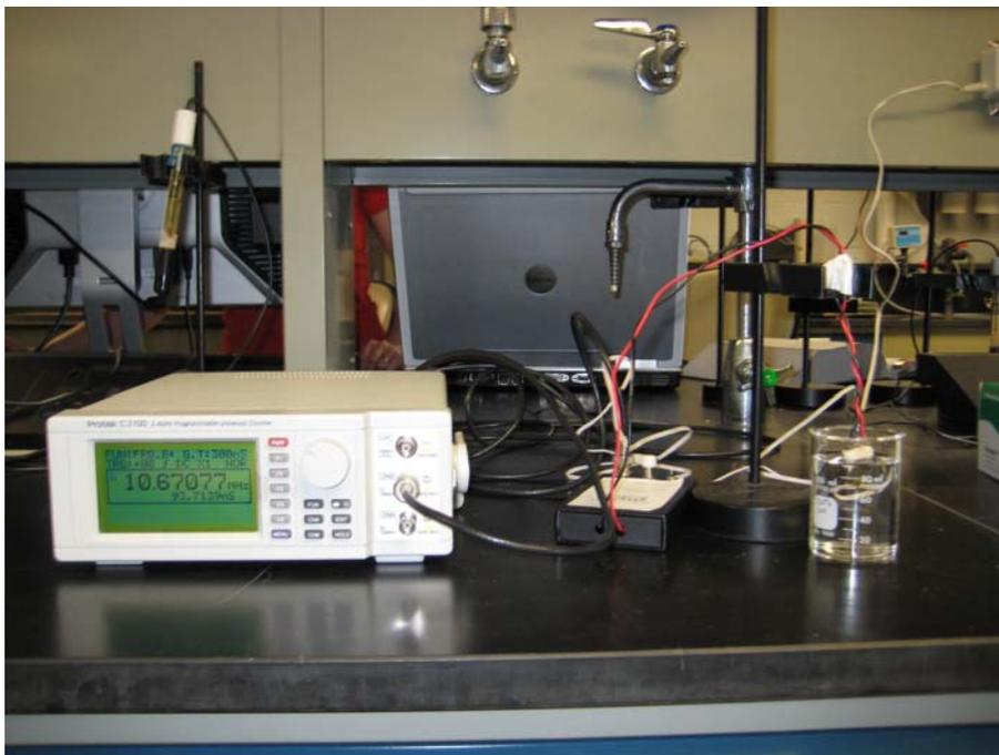
**Fig. 3 Lab Setup of Quartz Crystal Microbalance**
