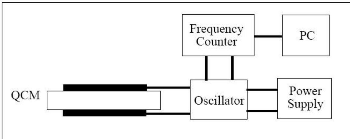
Fig. 2 Schematic Representation of the Mass Measurement Circuit
