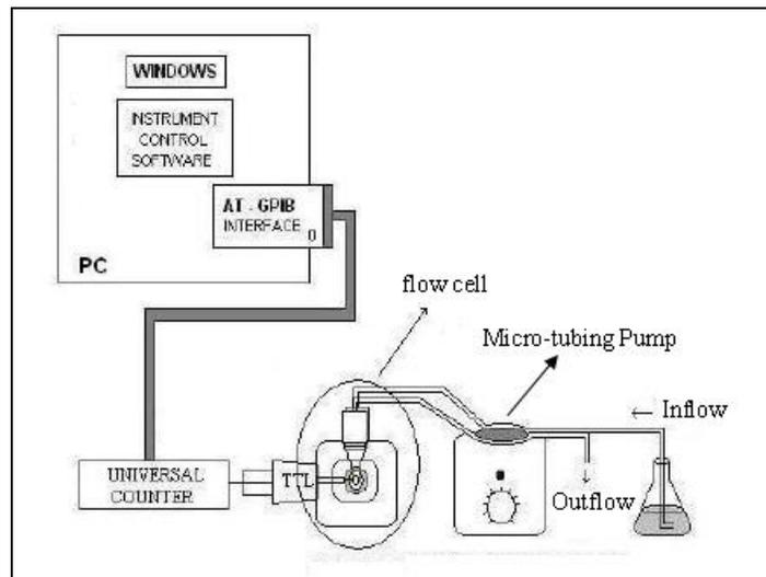
**Fig. 8 Experimental setup with flow cell (Adapted from Talib, 2006 with modification)**
