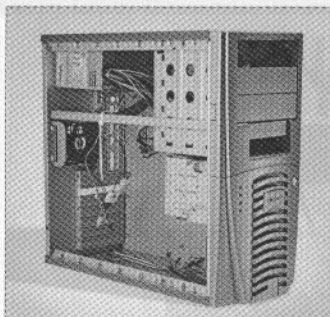
Choose a chassis that has a 300- to 400-watt power supply and leaves room for growth.
