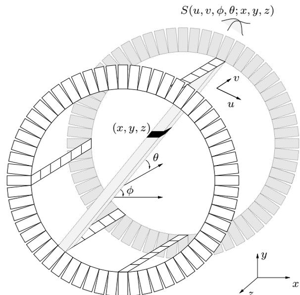
Fig 1. Illustration of fully characterized system response function,  $S$ , where  $(u, v)$  defines the point on one detector surface where the coincident bin with azimuthal and axial angle  $(\phi, \theta)$  intersects. And,  $(x, y, z)$  defines the location in the volume that contributes to this coincident bin.
