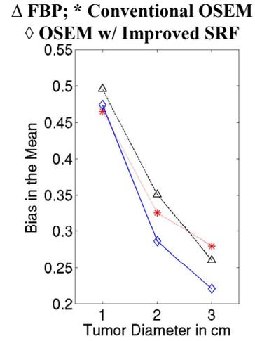
Fig 7. Plot shows biases in the mean values of all the tumors in unsmoothed reconstructions of noise-free data versus tumor size (standard error on these points range from 0.05 to 0.06). The OSEM w/SRF method does not improve the 1cm spherical lesion bias, but does improve the bias of 2cm and 3cm lesions by ~15%.
