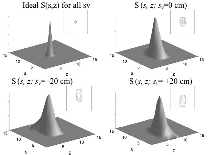
Fig 2.  $S_{3\text{DImproved}}(s, z; s_v)$  at several radial locations for a transaxial FOV[-27.5cm, 27.5cm]. The inlaid  $(s, z)$  contour plots mark the center of the ideal with a cross and show the half, fifth and tenth maximum contours.
