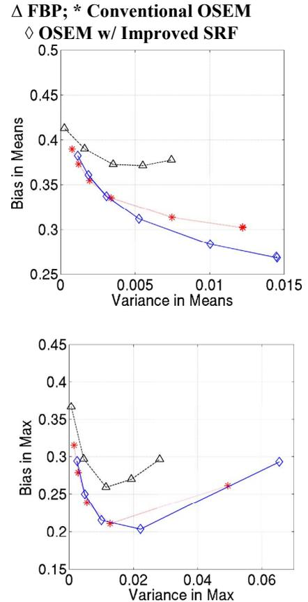
Fig 8. Analysis of quantitative accuracy of the OSEM w/SRF. Each datum point generated from reconstructions of 50 noise realizations. Top plot shows the mean of the bias of the mean values of each tumor region versus the variance in these mean values. Bottom plot shows the mean of bias of the max values of each tumor versus variance of max values. Each curve formed from varying the smoothing parameter of the reconstruction algorithm.
