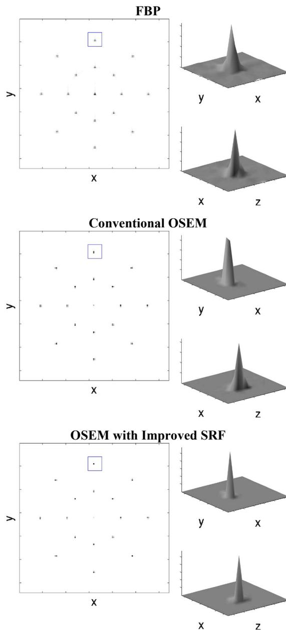
Fig 3. Reconstructions of simple phantom with point sources at 0cm, 10 cm and 20cm from center of FOV. Two surface plots show transaxial and axial slices through a single point. Our proposed method leads to reconstructions with improved resolution.
