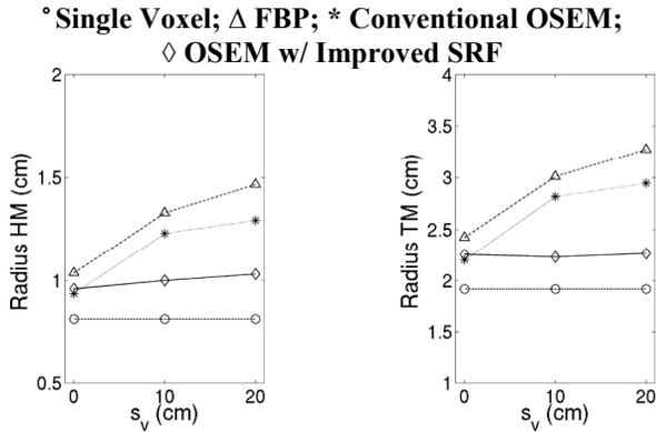
Fig 5. Presents volumetric figures for resolution analysis. Plots the average radius of a sphere inscribed in the half maximum and tenth maximum of each point source. Note the consistent resolution of the OSEM w/ improved SRF method throughout FOV
