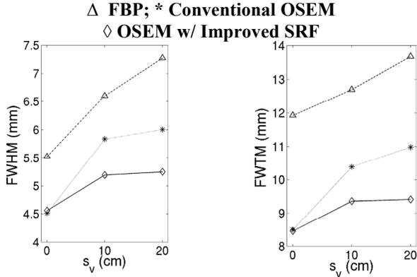
Fig 4. Average transaxial full width half maximum and tenth maximum of the reconstructed point sources. Note that our proposed method yields an ~10% improvement in resolution over conventional OSEM at locations away from center of FOV.
