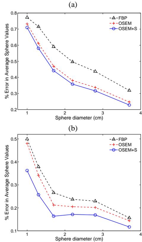
Fig. 7. Quantitative accuracy of each feature in the NEMA IEC Body phantom plotting the error in the average of voxels inside the spheres versus sphere size. Plot (a) is formed from images regularized with 10mm post-smoothing and (b) from images regularized with 2.5mm post-smoothing.
