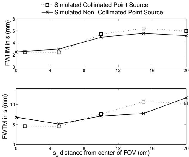
Fig. 1. FWHM and FWTM of  $S(s; s_v)$  formed from non-collimated and collimated point source at different locations.
