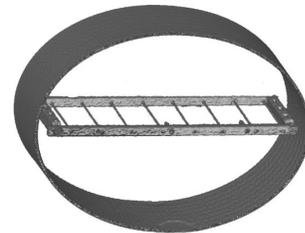
Fig. 8. Volume rendered image of CT scan of line source phantom showing the 8 line sources supported by a plastic frame.
