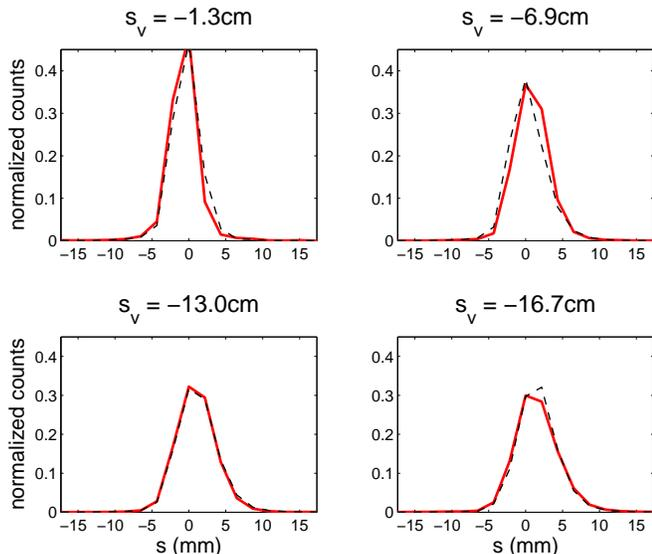
Fig. 4. Measured system response in  $s$  to Na22 point source positioned at 4 locations,  $s_v$  shown in solid line. The parameterized version shown in dotted line.
