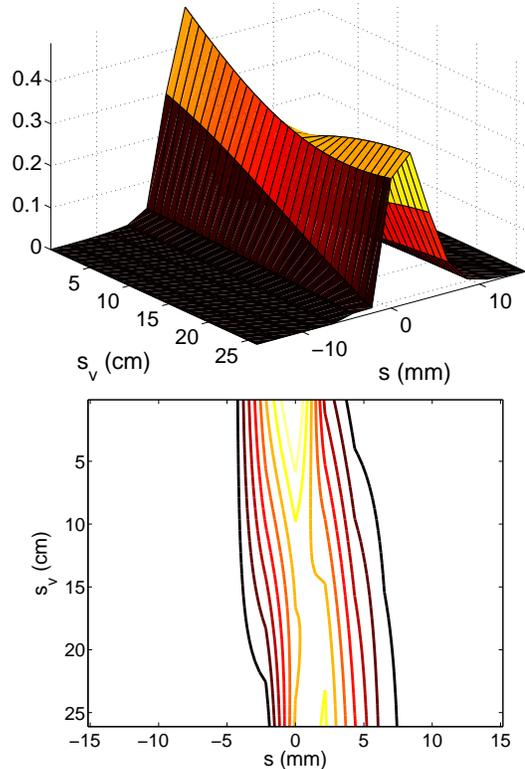
Fig. 5. Mesh and contour plot of complete  $S(s; s_v)$  for 0 to 25 cm from the center of FOV formed from parameterizing the measured  $S$  values and completing the function for all radial positions  $s_v$ .
