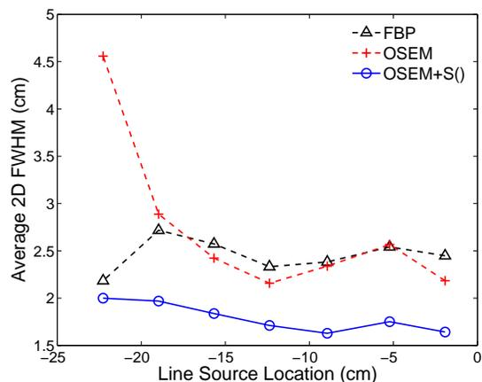
Fig. 11. FWHM versus line source location computed from images in figure 9
