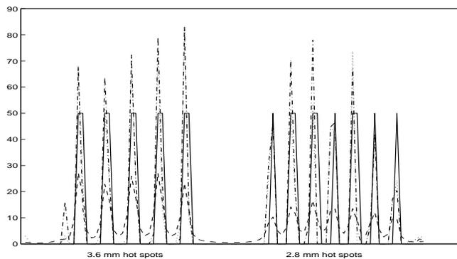
Fig. 2. Central portion of horizontal line 73 from simulated phantom. Reference image (solid), EM (dashed), Poisson MAP (dashdot), MAP-D (dotted)
