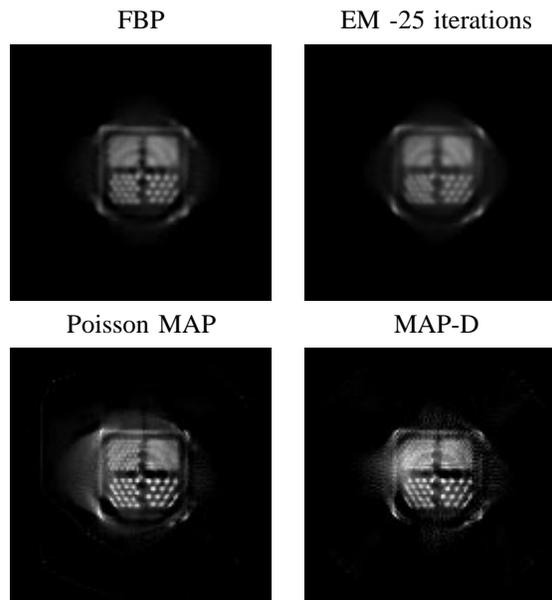
Fig. 3. 128x128 Reconstructions of Real Derenzo-like phantom from FORE rebinned 279x360 data. Consists of 4 quadrants with 4.0 mm diameter hot spots to 1.6 mm hot spots.
