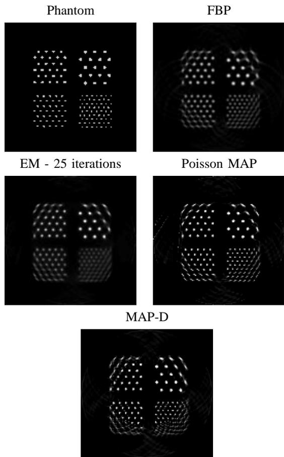
Fig. 1. 128x128 Reconstructions of Simulated Derenzo-like phantom from FORE rebinned 279x360 data. Consists of 4 quadrants with 5.6 mm diameter hot spots to 2.8 mm hot spots.
