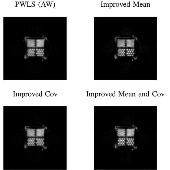
Fig. 3. One transaxial slice of  $128 \times 128$  reconstructions of Derenzo phantom
