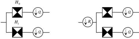
Fig. 2. Building blocks of the DFB (synthesis part). *Left*: quincunx filter bank required for the first two levels. *Right*: resampling followed by the quincunx filter bank required for levels three and higher.
