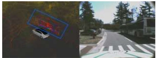
Figure 3. Example of dynamic changes of the environment. The points inside the blue bounding box in the left figure correspond to the passing bus in the right figure.
