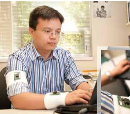
ECE graduate student Bo Dong wears a prototype of a new wearable sensor network.
