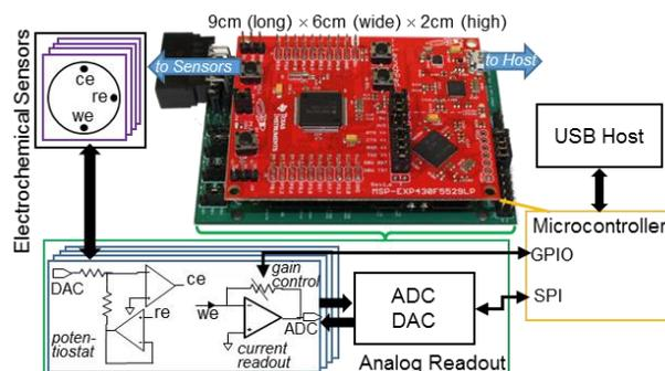
Fig. 1. Versatile electrochemical instrument for interfacing with a variety of electrochemical sensors and streaming measurements to a USB host.
