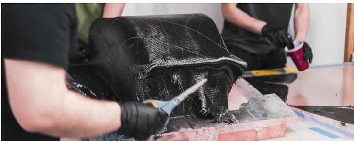
The left side-pod, an aerodynamic component, is laid up with carbon fiber
