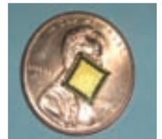
The low-cost, self-powered sensor is smaller than Abraham Lincoln's face on a penny.
