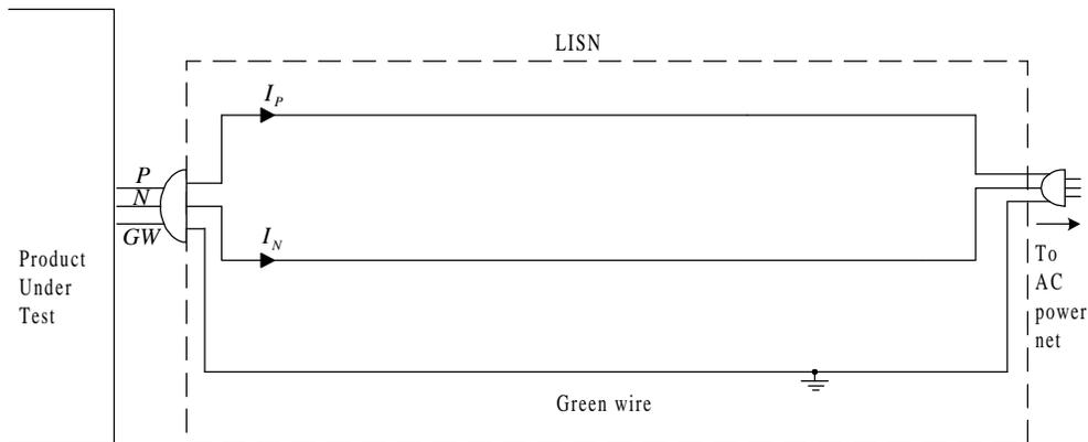
Thus the product under test will operate as if there were nothing between it and the ac power net at 60 Hz. In the frequency range of conducted emissions (450 kHz-30 MHz), however, the conductors will look like short circuits and the inductors will look like open circuits. The equivalent circuit will look like this:
