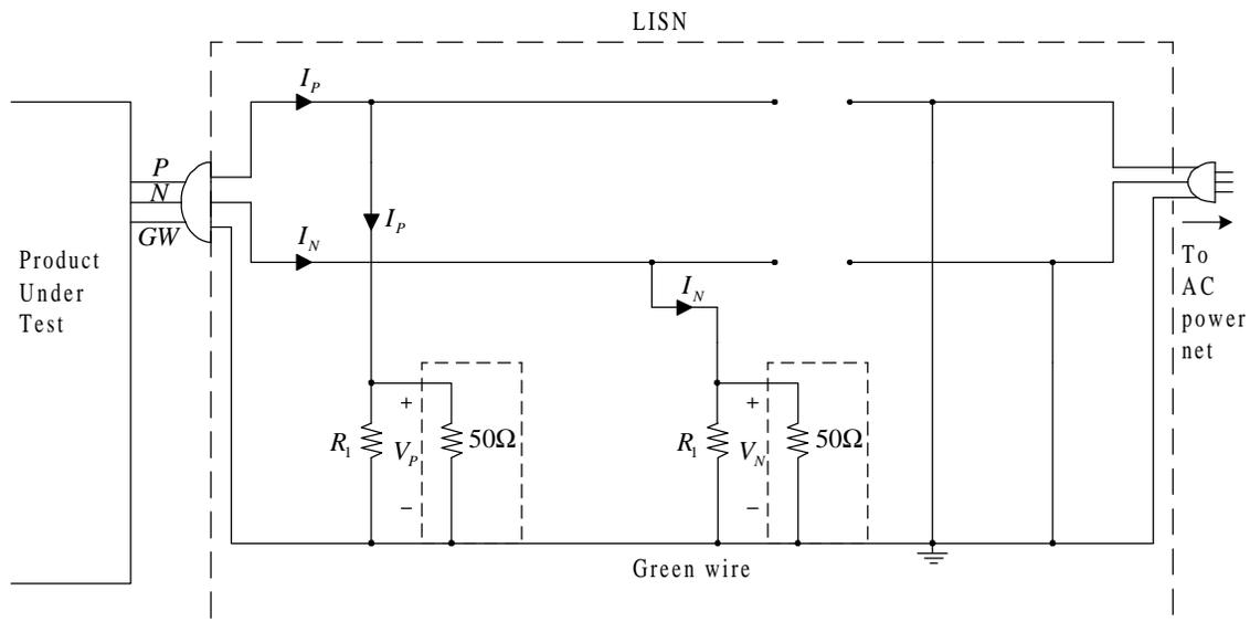
Thus, the currents on the neutral and phase lines can be isolated and measured at the  $50\ \Omega$  resistors. Notice that the currents on the phase and neutral lines have no path that they can get onto the ac power net with.
