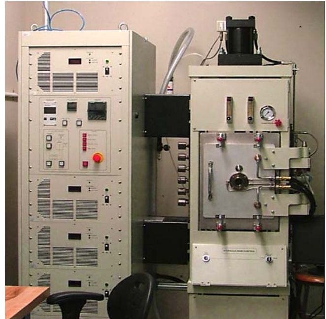
FIGURE 1. Pulsed electric current sintering system for densification of thermoelectric materials.
