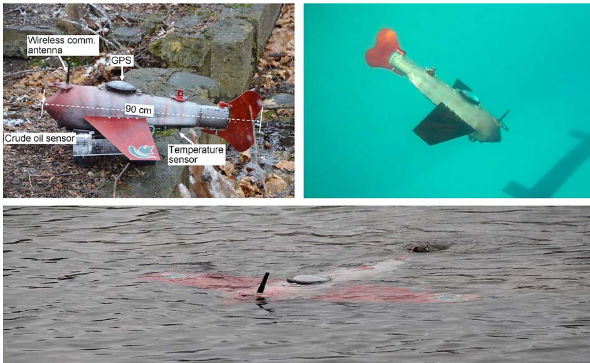
FIGURE 3. Gliding robotic fish “Grace” developed by SML: (top, left) Dimensions and equipped sensors; (top, right) the robot demonstrating gliding in a pool; (bottom) the robot swimming in the Kalamazoo River and sampling crude oil concentrations.
