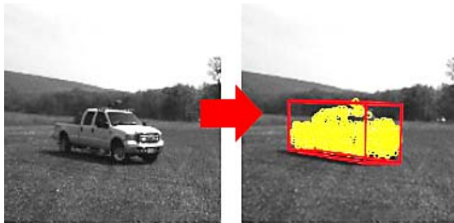
FIGURE 1. 3D LIDAR points on a nearby vehicle enable automatic vehicle pose estimation.
