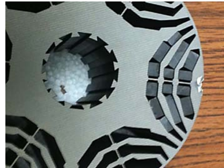
FIGURE 3. PMASynRM stator with ferrite magnets.
