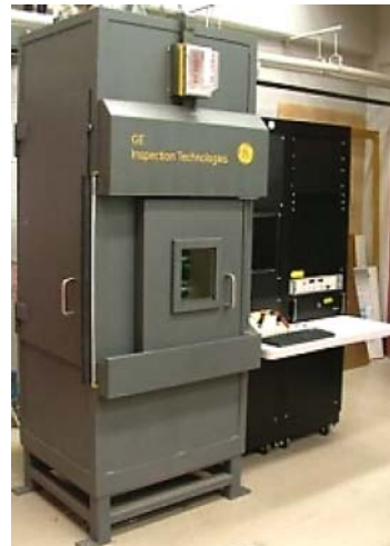
FIGURE 6. GE vertical x-ray inspection system with high precision rotation stage ( http://www.egr.msu.edu/erc-cleanroom/equipment/xray/index.php )
