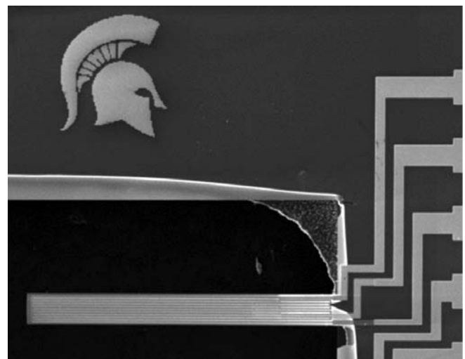
FIGURE 1. Top: \text{VO}_2 -based MEMS actuator chip design. Mr. Rafmag Cabrera (graduate student) holding wafer. Bottom: Fully suspended MEMS actuator with patterned resistive heaters.
