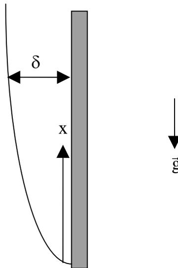
As the boundary layer thickness grows, the fluid mechanics change significantly, so that the convective heat transfer coefficient will vary along the length of plate and we will have a local convective heat transfer coefficient,  $h_c(x)$ . Then we may also define local Nusselt and Rayleigh numbers as
