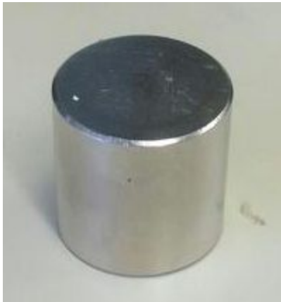
Fig. 3.1 - Neodymium magnet used for inducing fields
