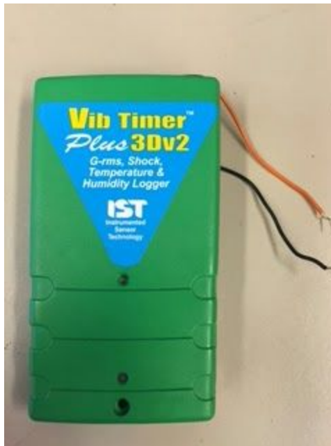
Figure 3.13 - Replaced power system for VTP-3Dv2.
