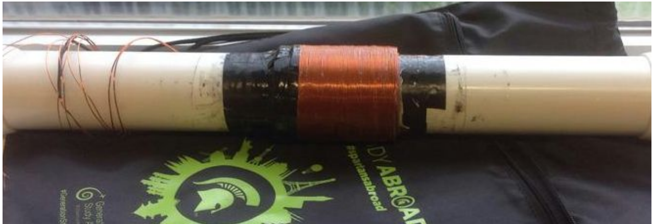
Figure 3.6 - Inductor coil for harvesting
