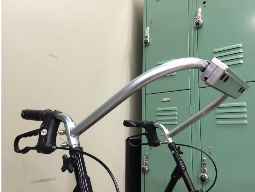
Figure 3.2.3.3: Fabricated Crossbar and Housing
