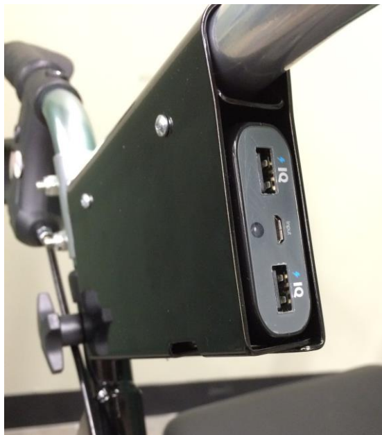
Figure 3.4.3.6: Anker Power Supply in Housing
