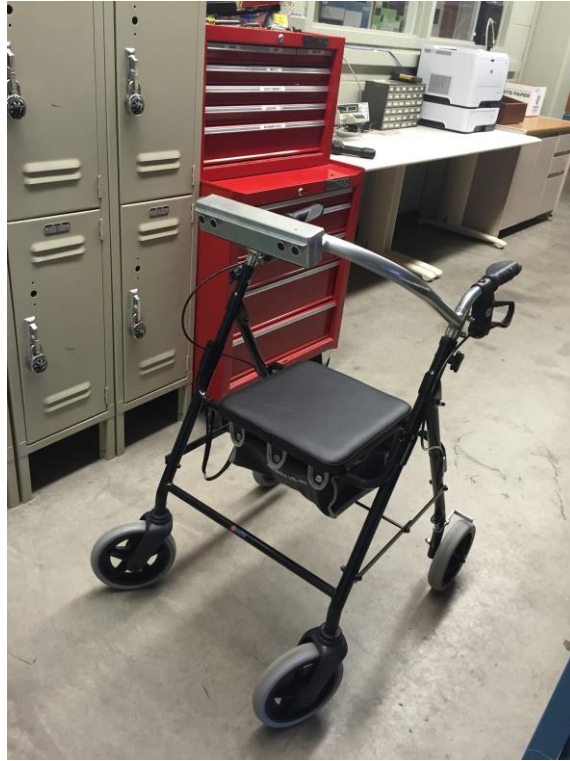
Figure 3.2.3.1: Fabricated Housing on Walker
