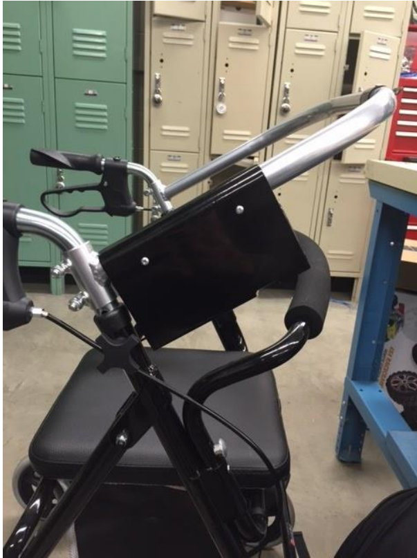
Figure 3.4.3.4: Power Supply Housing
