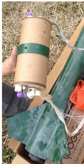
Figure 4.4.1 The Madcow Torrent after its launch. The purple objects are the undeployed charges.
